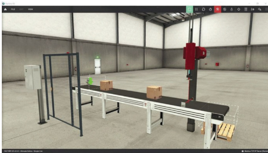
Figure 5.16 Process in FactoryIO controlled from OpenPLC.
