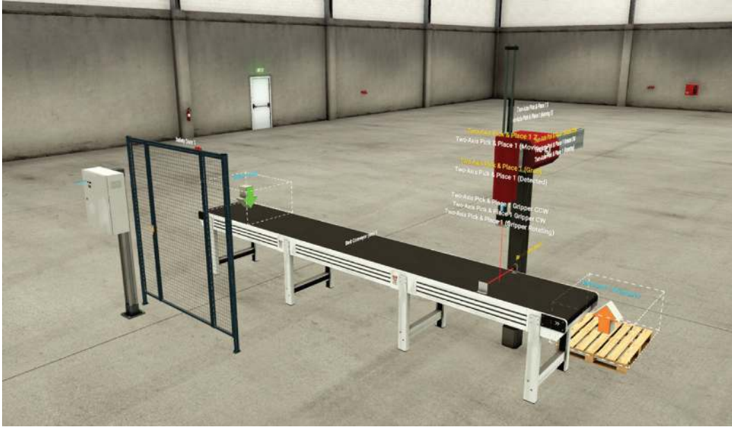
Figure 5.7 Placement of elements in the FactoryIO scene.
