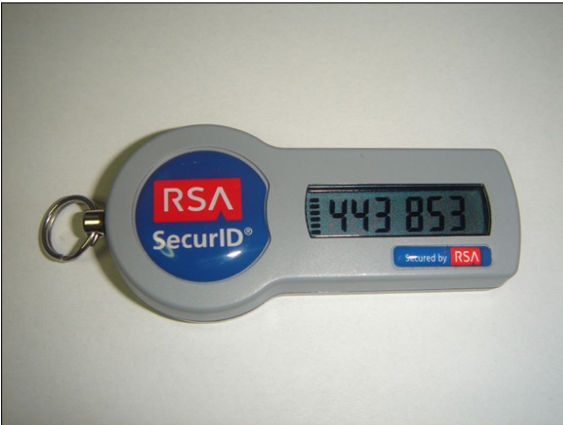
FIGURE 8-4: An RSA SecureID brand one-time password generator hardware token.
