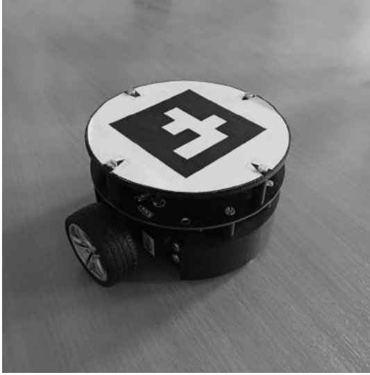
Figure 6.10: Assembled Mechalino with ArUco marker on top. ↵
