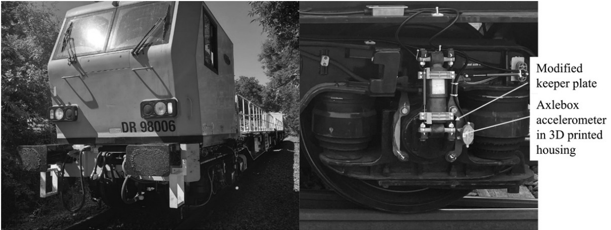
FIGURE 5.42 MPV and sensor installation on the axlebox and across the primary suspension. ↗
