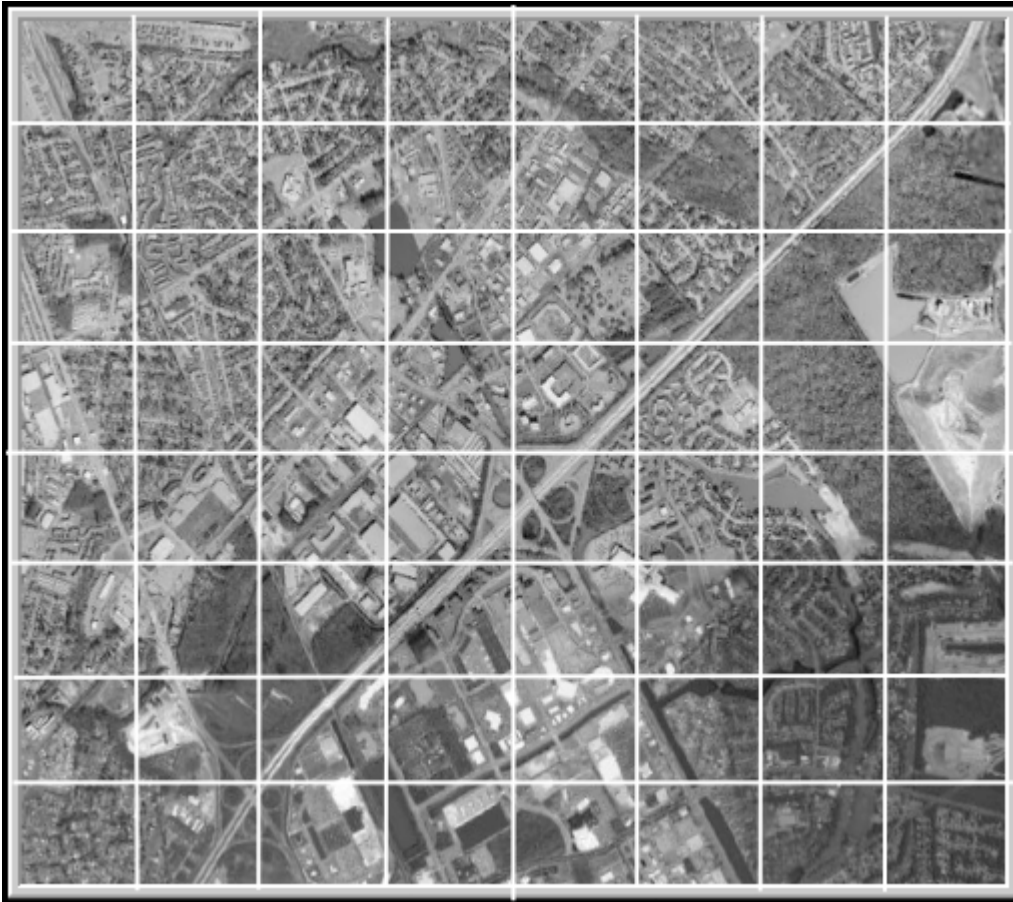
FIGURE 5-1: A grid overlay shows how each square represents a portion of real geographic space.
