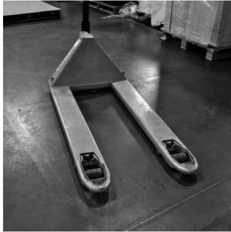
FIGURE 2.5 Hand-pushed pallet transporter. This may look harmless, but the small, hard tyres are hard on floor joints.
