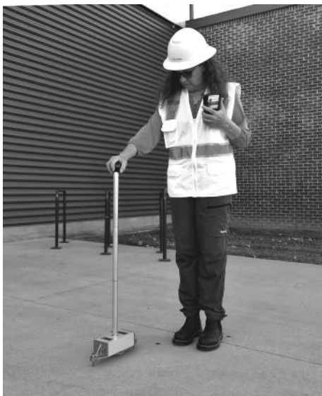
FIGURE 20.4 Measuring surface regularity with a walking profiler. The operator walks it over the floor in a straight line, pivoting on the front foot after each step. The result is a connected series of elevation differences measured on 300-mm (12-in) centres. The data can be analysed to determine F_F , F_L , and F_{min} .
