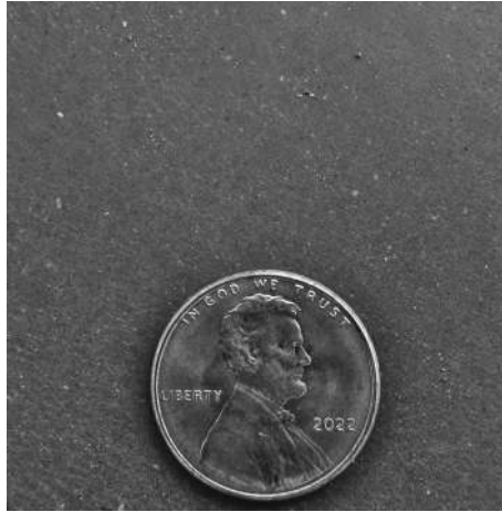
FIGURE 18.10 Burnished finish. This is the smoothest finish achievable by trowelling. The coin, for scale, has a diameter of 19 mm.
