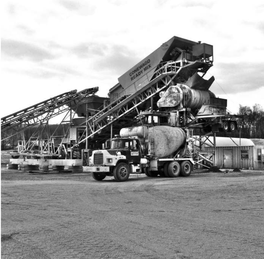
FIGURE 9.1 This mobile batch plant has all the capabilities of a fixed plant but can be taken apart and moved between jobs.
