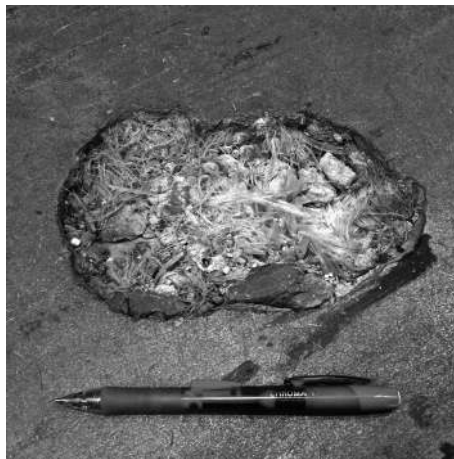
FIGURE 12.6 These polypropylene fibres (macrosynthetic) tangled and formed a ball. Any type of fibre can tangle, but the risk is higher when the fibres are long and thin.
