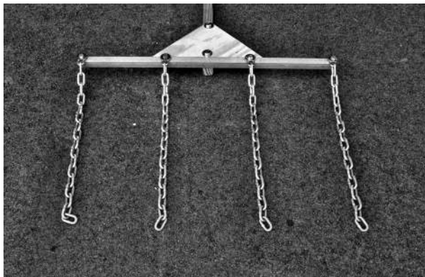
FIGURE 19.3 The chain-drag tool for finding delaminations.
