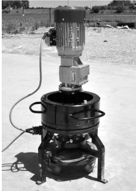
FIGURE 21.1 Chaplin abrasion tester.
