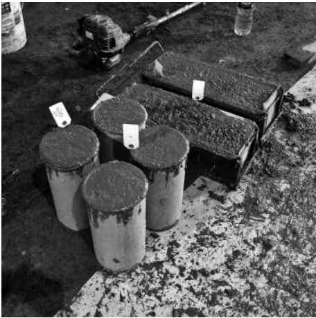
FIGURE 7.1 This sample includes cylinders for compressive strength and beams for flexural. Most of the world uses cylinders for compressive strength, but the UK uses cubes.
