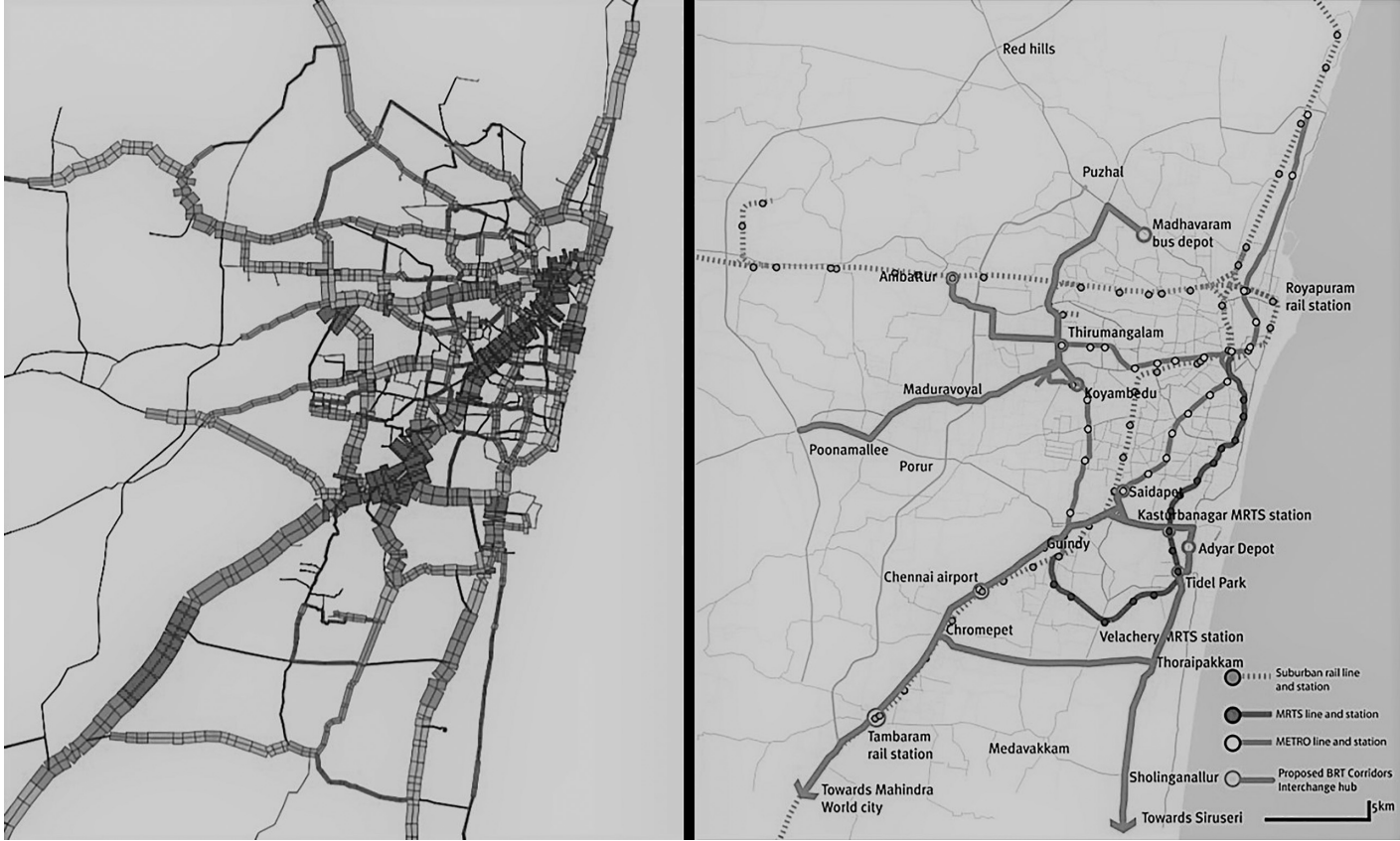
FIGURE 10.10 Correspondence between the choice of rapid transit technologies and the expected level of demand (left)
