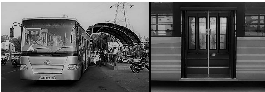
FIGURE 10.6 The Janmarg system in Ahmedabad, India, with doors on either side of the rapid transit bus
