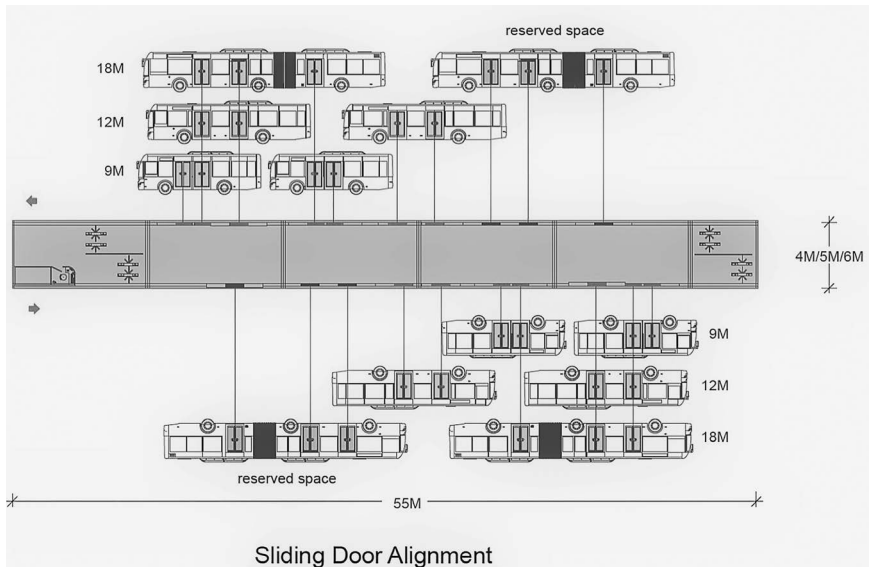
FIGURE 10.21 Alignment of bus and station doors designed to accommodate all types of vehicles
