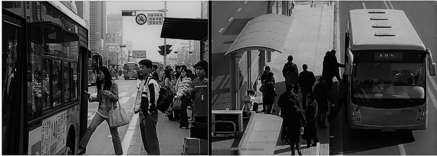
FIGURE 10.4 Lack of level boarding and onboard fare collection in Seoul, South Korea
