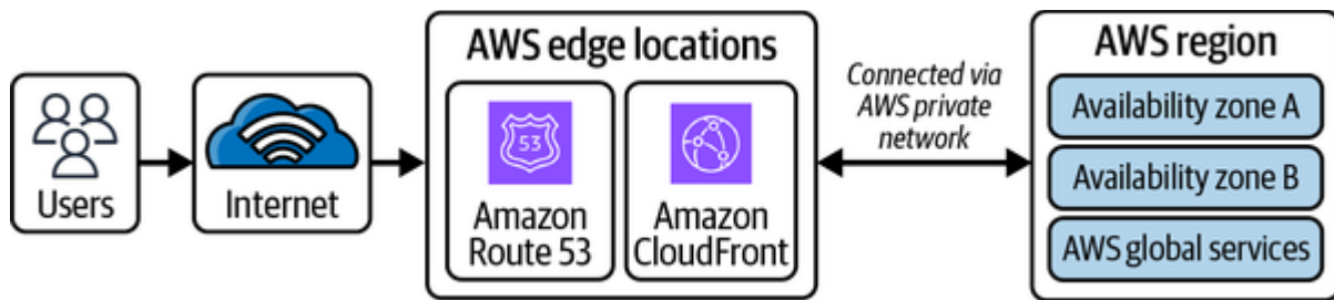
Figure 9-1. Connectivity to an AWS region via an edge location
