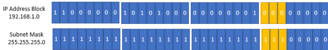
Figure 6.12 – Creating subnets by borrowing bits from the host portion of the IP address
