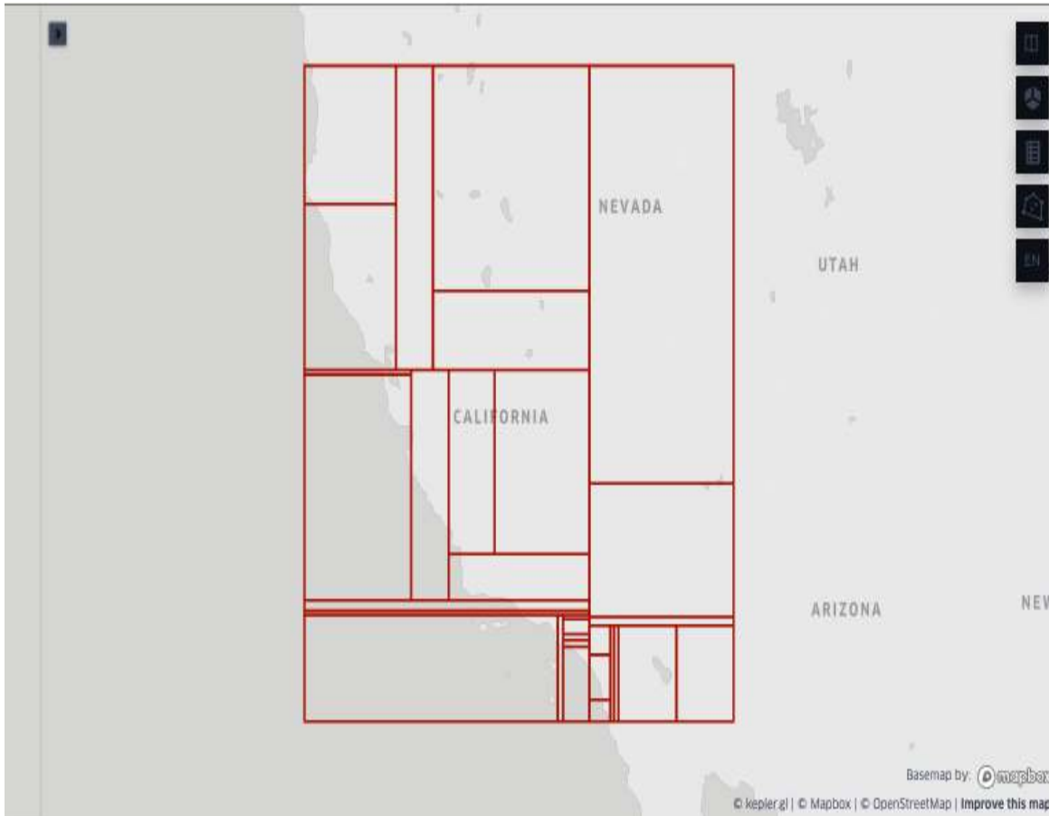
Figure 10-2. In KDB-based partitioning, partitions have no overlaps
