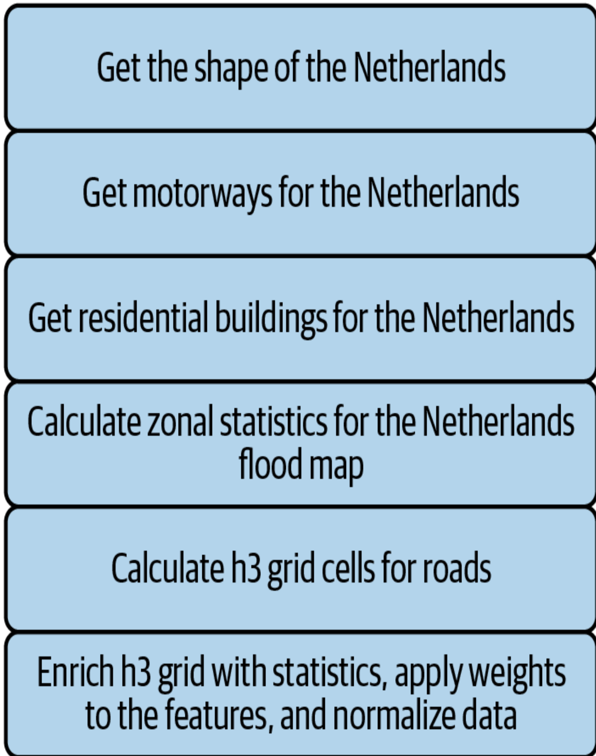
Figure 8-7. Process of creating a data product utilizing the geospatial lakehouse architecture
