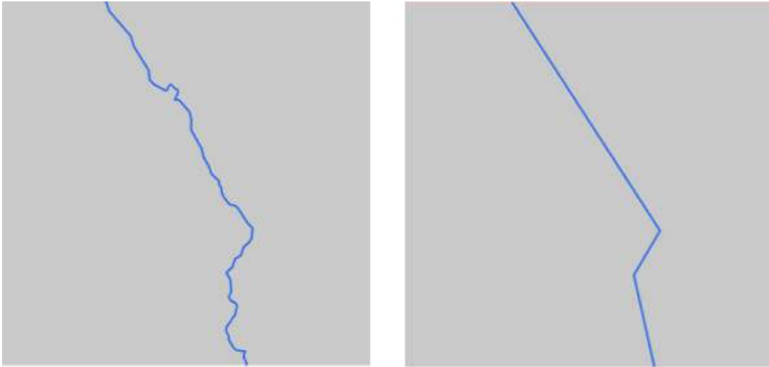
Figure 4-9. Result of the ST_Simplify function on the linestring geometry: on the left is an input geometry, and on the right is the output
