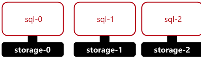
Figure 1-2. An example StatefulSet – each Pod has a unique, ordered, and persistent name. Each Pod also has persistent storage associated
