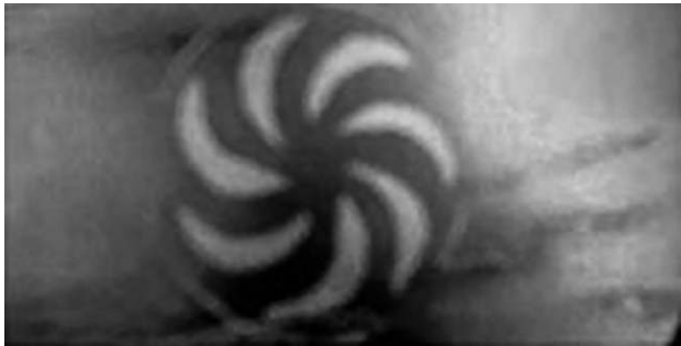
FIGURE 12.12 Image recording in the LC polymer film induced by temperature and UV irradiation.
