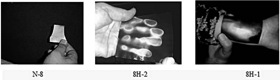
FIGURE 12.13 Image recording in the polymer film induced by temperature.
