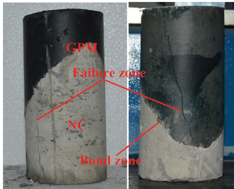
FIGURE 5.20 Typical failure modes of GPMs.
