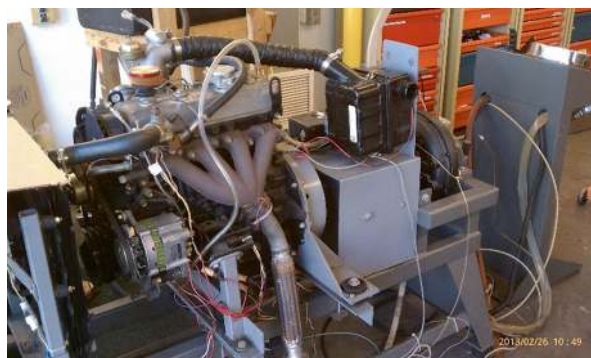
Fig. 13.4 Isuzu 4-cyl 1.9L diesel engine modified for operation on dimethyl ether undergoing tests on dynamometer, at California Polytechnic State University. Photo by author
