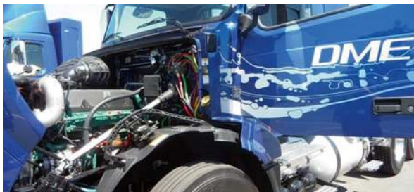
Fig. 13.11 Volvo DME truck engine, 2013. Uses a relatively low-pressure common-rail injection system as described in text. From https://www.truckinginfo.com/152918/volvo-thinks-the-fuel-of-the-future-is-dme-and-its-almost-here . With permission
