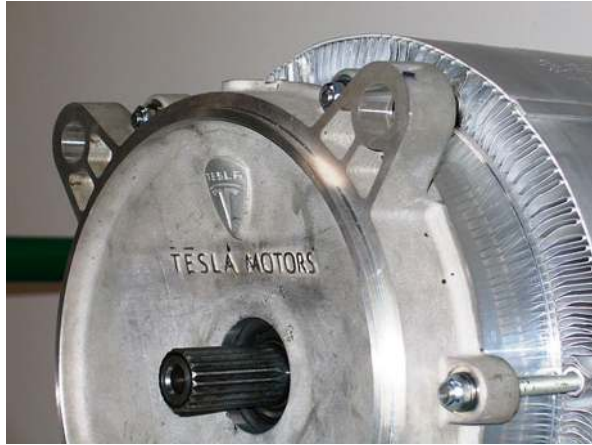
Fig. 14.43 185 kW air-cooled induction motor used in the Tesla Roadster. Image by Tesla Inc., 31 December 2015, copied from https://fuel-efficient-vehicles.org/energy-news/?page_id=1065 Public domain.
