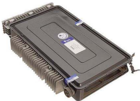
Fig. E.8 Typical engine control module (ECM) that handles both fuel and ignition control. Photo unattributed
