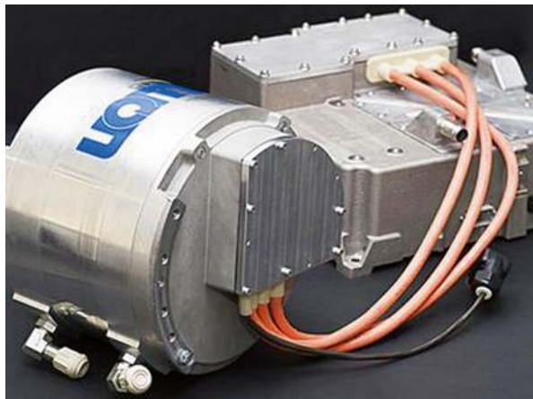
Fig. 14.40 UQM (formerly Unique Mobility) electronically commutated permanent magnet EV motor and drive electronics. UQM HDPP100 100kW Drive System. Image from Unique Mobility, early 1990s, https://www.thunderstruck-ev.com/uqm-pp100-coda.html DIY EV parts exchange. Public domain
