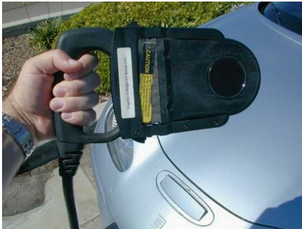
Fig. 14.18 GM/Delco Magne-Charge inductively coupled EV charge paddle. Shown in front of a 1998 GM EV-1 that used this charging method exclusively. Image from Renewable and Sustainable Energy Reviews. Publisher: Elsevier. https://www.researchgate.net/publication/309666212_00005361_125788 Used under STM guidelines
