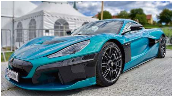
Fig. 14.29 The 2022 Production Land Speed Record holder, the Rimac Nevara. 1914 HP, 256 mph (412 kph) maximum speed, 0–300 kph acceleration in 9.22 s, 120 kWh LiMgNiCo battery, undisclosed weight. Capable of speeds four times the US freeway speed limit and more expensive than some luxury yachts.
