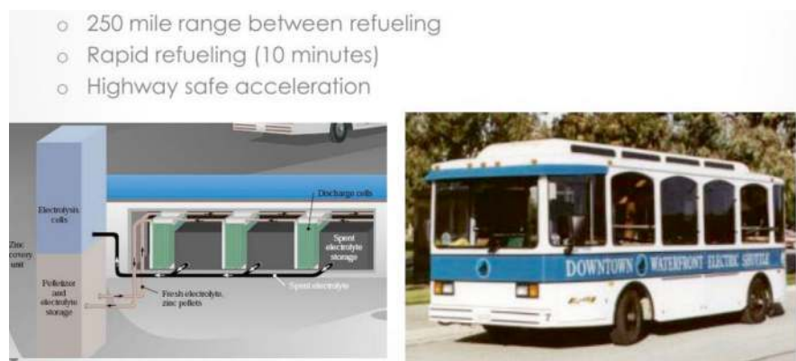
Fig. 14.60 Zinc-air batteries were used experimentally in one of the Santa Barbara Downtown shuttle buses in 2011. From Marta Baginska “Metal-Air Batteries: Types, Applications, and Challenges,” NPRE 498 Energy Storage Systems 12.07.2011. Mar 13, 2019. Public domain
