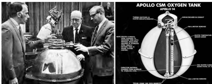
Fig. 9.24 Redesigned liquid oxygen tank used on NASA moon landing missions following the explosion of a liquid oxygen tank on Apollo 13. NASA photos, public domain
