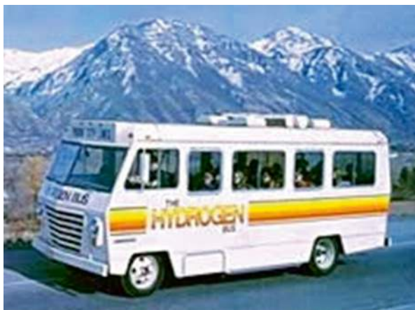
Fig. 9.12 Winnebago shuttle bus modified to run on compressed hydrogen by Billings Energy Research, possibly as early as 1976. Photo and information from https://www.rogerebillings.com/1976-the-hydrogen-bus/ . Public domain
