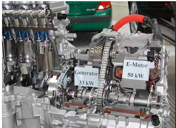
Fig. 15.13 Gen 1 (1997) Toyota HSD transmission cutaway showing MG1 (labeled generator), MG2 (labeled E-motor) and planetary gearset between them in common housing. Noncopyrighted photo, posted on user forum https://www.yarisworld.com/forums/showthread.php?t=10424&page=6
