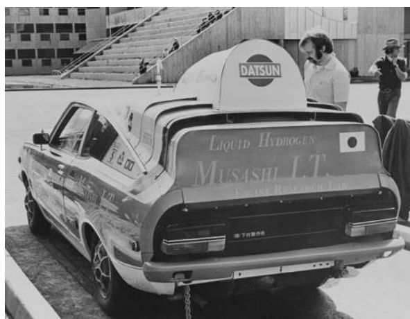
Fig. 9.10 Liquid hydrogen converted Datsun B210 constructed by students at Musashi Institute, Japan. Photo from the 1975 SEED (Student Engineered Economy Design) Rally. Public domain
