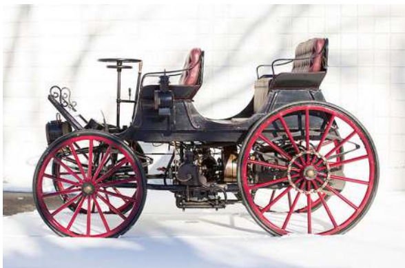
Fig. 15.18 Believed to be the first petrol/electric hybrid vehicle, the 1896 Armstrong Phaeton was produced in small numbers by the American Horseless Carriage Company in the USA. Photo from Hemmings Motor News, https://www.hemmings.com/stories/perhaps-the-worlds-first-hybrid-an-1896-armstrong-sells-for-483400-at-amelia-island/ with permission
