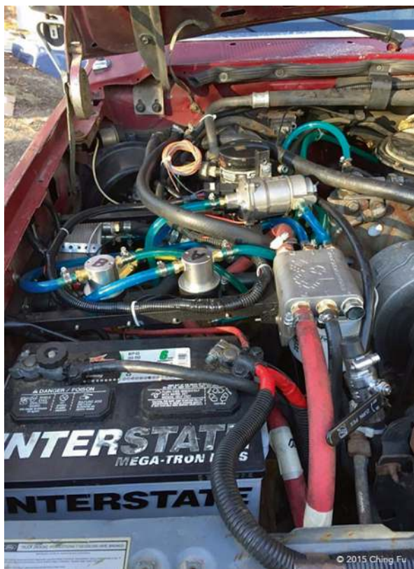
Fig. 16.8 Underhood view of DIY greasel conversion of a 1987 Ford F350 diesel truck. From https://www.livesmallridefree.com/blog/wvo-101-waste-vegetable-oil-vehicle-basics . With permission
