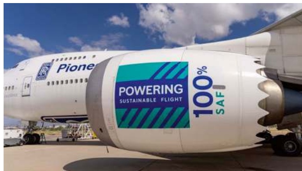
Fig. 11.5 Rolls Royce Trent 1000 engine modified to run on 100% sustainable aviation fuel. Image copyright Rolls Royce Ltd., https://www.adsadvance.co.uk/rolls-royce-joins-boeing-and-world-energy-for-successful-100-saf-flight.html . With permission
