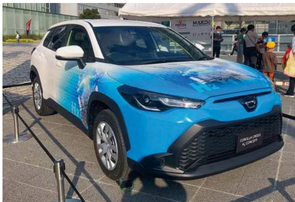
Fig. 9.75 Prototype of Toyota Hydrogen ICE Hybrid Corolla, announced in 2022. Photo by KKPCW (Kyu3) in Nagoya, Japan, 2022-10-23.
