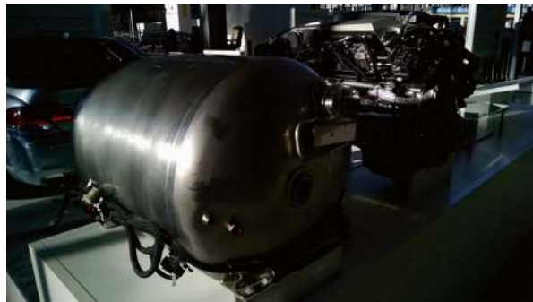
Fig. 9.16 Linde Liquid hydrogen tank used by BMW in 750i hydrogen conversion of Fig. 9.17. Deutsches Museum, Munich, Germany. Photo: author, 2016
