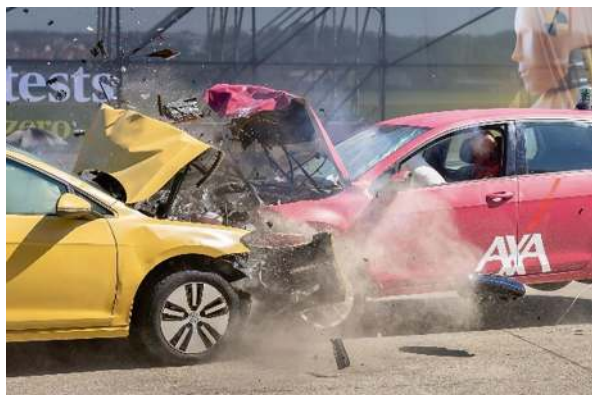
Fig. 14.71 Frontal crash test conducted by the Swiss insurance company AXA, between two nearly identical 2022 Volkswagen Golfs, one an ICE model, the other an EV model. Guess which one is the EV? (the yellow one on the left). Photo by Michael Buholzer/AXA. Unrestricted use
