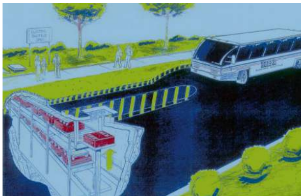
Fig. 14.88 Rapid Battery Interchange (RBI) for transit buses, “Coke machine” Concept. Developed for the California Energy Commission and Pacific Gas and Electric Co, 1991
