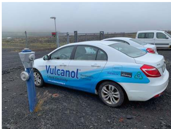
Fig. 11.3 Vulcanol is the trademarked name for e-methanol produced by Carbon Recycling International's CO 2 -to-fuel process in Iceland. Uses geothermal electricity to produce electrolytic hydrogen, then methanol synthesis using CO 2 from atmospheric carbon capture. Vehicle is a 2020 Geely Emgrand methanol sedan produced for the Chinese market. Image copied from Damien Speight, Nature's recipe for a world run entirely on green energy: Green Carbon & Renewable Fuels . Original photo by Zhejiang Geely Holding Group Co Ltd. Public domain
