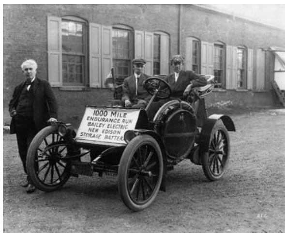
Fig. 14.8 Bailey Electric Runabout equipped with Edison batteries after 1000 mile trip across England, 1911. Thomas Edison NHP archive. Public domain
