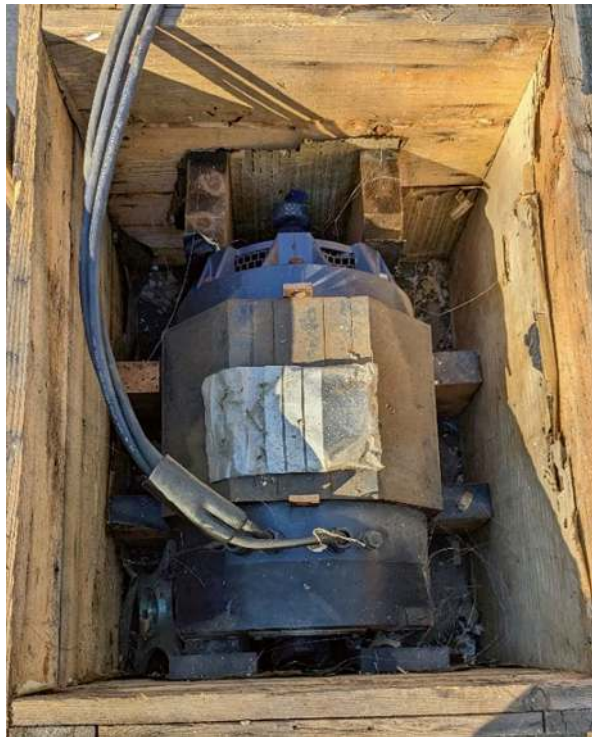
Fig. 14.33 The Nelco N200L, a durable series-wound brush-commutated motor. Prior to approximately 1995 it was the most widely used motor for small-to-medium capacity electric buses and shuttles. The motor in this photos is a NOS replacement part for a 1989-1992 GM/Conceptor electric G-Van. Photo:author
