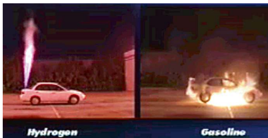
Fig. 9.58 Demonstration of a hydrogen vs gasoline vehicle fire. DOE-funded 2001 demonstration conducted by Michael Swain at the University of Miami in Florida, USA. Photo from https://ecv.hyundai.com/upload/newsroom/BL00200514/Green-Tech-010-Is-Hydrogen-Safe-Sep2023.pdf . US DOE copyright in public domain
