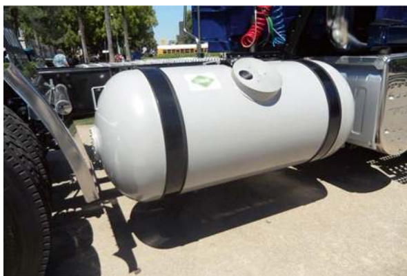
Fig. 13.10 DME fuel tank on Volvo Class 7 truck. Same specifications as an LPG tank, with 125 psig working pressure, 250 psi maximum pressure. https://www.truckinginfo.com/152918/volvo-thinks-the-fuel-of-the-future-is-dme-and-its-almost-here . With permission
