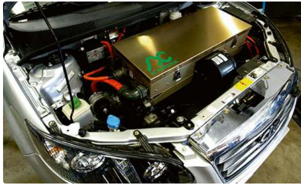
Fig. 14.50 AC-150 (200 HP) Power Controller Unit by AC Propulsion of San Dimas, CA. shown installed in a 2007 AC Propulsion “e-Box”, a modified Toyota Scion xB minivan. Photo from http://www.acpropulsion.com/products-tzero.html . Photo taken at Cal Poly EV exhibition in 2007
