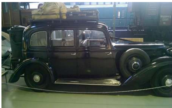
Fig. 16.4 1934–39 Adler Diplomat wood-powered limousine in Deutsches Museum, Munich, Germany. The large roof rack was used to carry extra wood chunks for the gasifier. Photo by author
