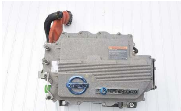
Fig. 14.49 Motor controller electronic assembly removed from a 2012 Nissan Leaf. Source: E-Bay “2011-2012 NISSAN LEAF EV INVERTER ASSEMBLY POWER HEAD” Accessed 1 December 2024
