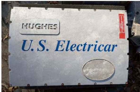
Fig. 14.51 Hughes Electronics 50 kW 312V Dolphin Controller, used in the U.S. Electricar electric S-10 light truck, 1994. Also used in upgraded 100kW form for the GM EV-1. Photo by author
