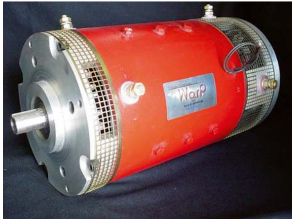
Fig. 14.35 The Warp 9.25" series-wound DC motor, rated at 32.5 HP continuous, but as much as twice for brief periods. Among the most popular motors for DIY EV conversions due to its lower weight compared with industrial electric motors. Photo found on http://rebirthauto.com/nmwarp9.aspx DIY EV parts exchange. Public domain.
