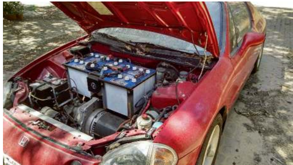
Fig. 14.19 Example of a DIY conversion of a 1994 Honda del Sol into an EV. It carried 18 eight-volt lead-acid batteries that nearly doubled the vehicle mass, compromising braking and steering. Photo by author
