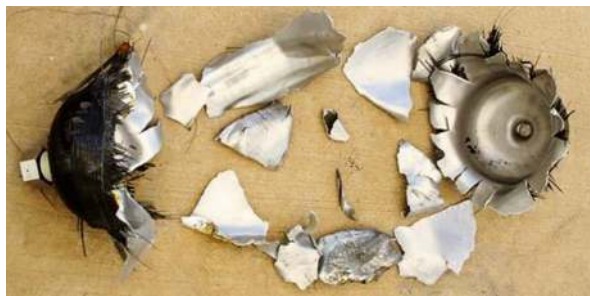
Fig. 9.35 Carbon fiber over aluminum high pressure cylinder after overpressure failure. From report by William P. Schonberg. Will it Leak? Will it Burst? COPV Perforation and Rupture after a MMOD Impact NASA publication, 2023. https://ntrs.nasa.gov/api/citations/20230012105/downloads/8-16-23%2020230012105.pdf . Public domain
