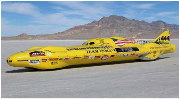
Fig. 14.26 Team Vesco 444 “Little Giant” Team Vesco 444, US EV Speed Record holder 2021, at 353 mph powered by 1152 prismatic lithium-ion batteries and heavily modified Tesla motors, 2021. Image from https://www.carscoops.com/2021/10/team-vesco-444-little-giant-broke-the-national-ev-record-with-353-mph/ Public domain
