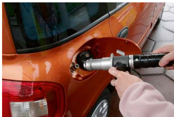
Fig. 8.6 Fast-fill dispensing of CNG at a refueling station. (From DOE AFDC. https://afdc.energy.gov/fuels/natural-gas-cng-stations . Public domain)
