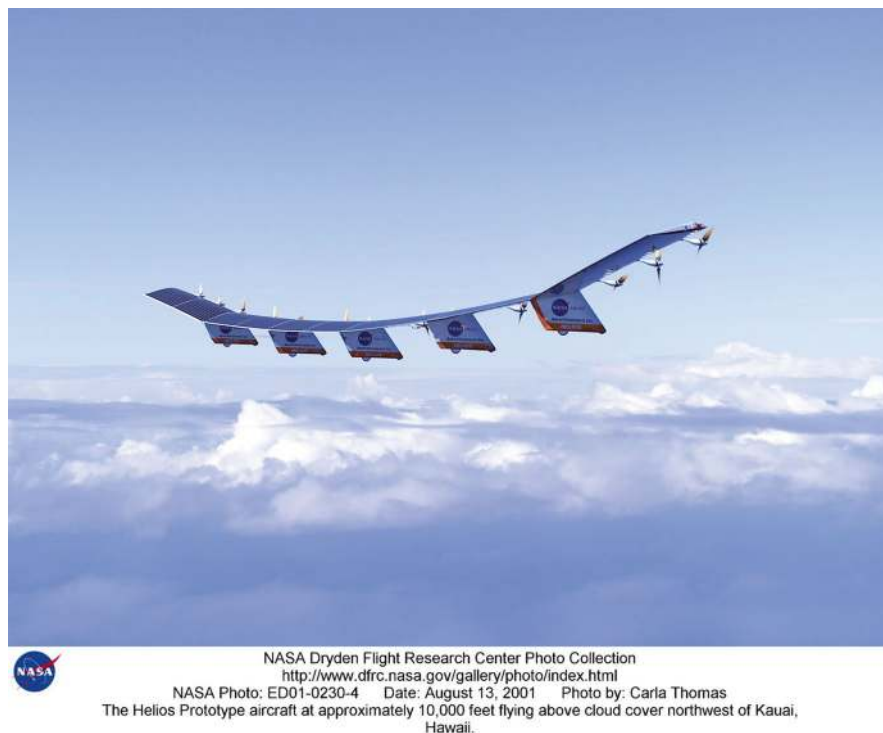
Fig. 9.42 2001 NASA photo of Helios remotely piloted ultralight aircraft, designed for nearly perpetual flight by use of solar/electric propulsion and reversible hydrogen fuel cells for storage of energy for night flight. https://ia601309.us.archive.org/27/items/NIX-ED01-0230-4/ED01-0230-4.jpg Public domain
