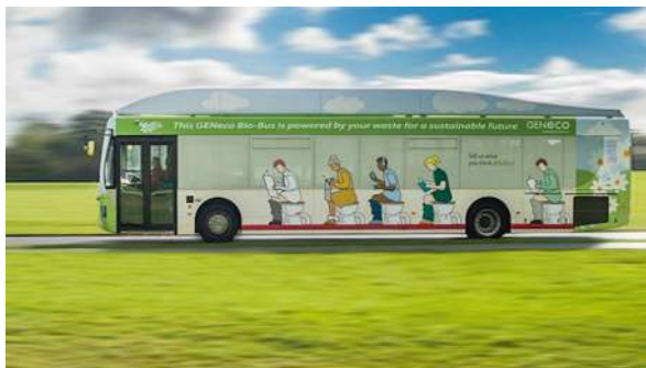
Fig. 16.9 Bristol City Bio-Bus, 2020. One of a city fleet of 77 biomethane-converted Scania buses. https://www.bioenergy-news.com/news/77-biomethane-powered-buses-launched-in-bristol-uk/ . Public domain
