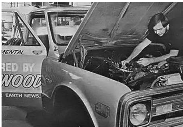
Fig. 16.3 1970s pickup truck converted to run on wood gas by Mother Earth News. Photo from 1981 Future Fuels Rally, a transcontinental alternative fuel competition. Used with permission
