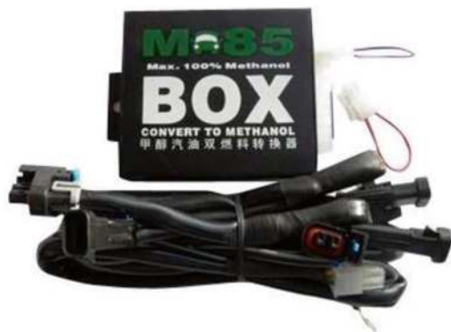
Fig. 6.9 Example of a low-cost aftermarket methanol conversion device that extends the fuel injection pulse duration to double the volumetric fuel delivery under any engine condition. The device works well except at high RPM when the maximum pulse duration may exceed the total allowable time for the injection of fuel in each complete engine cycle, which is two rotations of the engine. ( https://www.aliexpress.us/?spm=a1z5k.7633538.0.0.55565a870FymP9&gatewayAdapt=glo2usa . Public domain)
