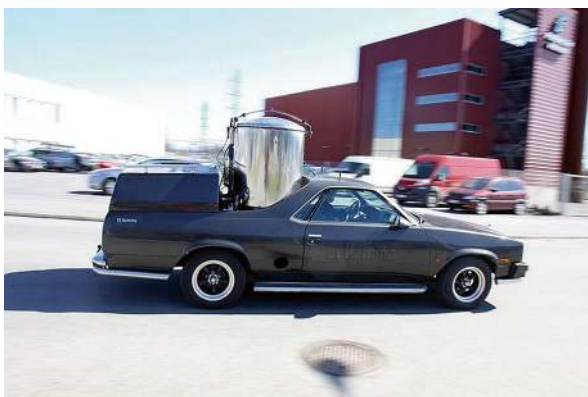
Fig. 16.6 Wood gas-converted 1987 Chevrolet El Camino, converted and owned by former (2015–19) Finnish Prime Minister Juha Sipilä. https://www.iltalehti.fi/autot/a/201206110100352#gallery . Public domain
