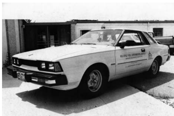
Fig. 6.10 Modified 1981 Nissan 200SX, capable of tri-fuel methanol/ethanol/gasoline operation. (Constructed by author in 1981 at the Denver Research Institute in Colorado under a DOE contract to demonstrate and compare multi-fuel operational characteristics. Photo: author)
