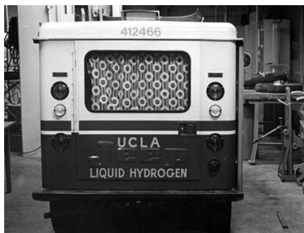
Fig. 9.9 The 1974/5 UCLA Liquid Hydrogen mail service vehicle. Built under contract to the US Postal Service as an evaluation platform. Photo: author, 1975
