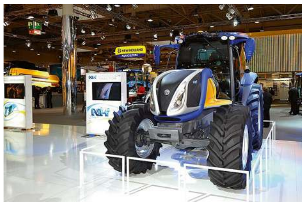
Fig. 9.14 New Holland prototype farm tractor powered by hydrogen generated onboard by reformation of ammonia. https://commons.wikimedia.org/wiki/File:New_Holland_NH2_hydrogen_tractor_at_Agritechnica_2009.jpg . CC Attribution-Share Alike 2.0 Generic license
