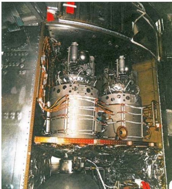
Fig. 9.23 Hydrogen-oxygen fuel cells in Apollo command module. NASA photo. Public domain
