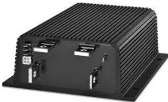
Fig. 14.48 Curtis 1204M PMC motor controller for golf cars and low-power electric vehicles. Photo: author
