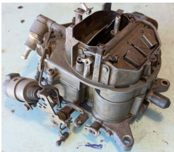
Fig. 4.5 Autolite 750 CFM 4-barrel carburetor from 1971 Ford 5.7L V8 engine. (Photo: author)
