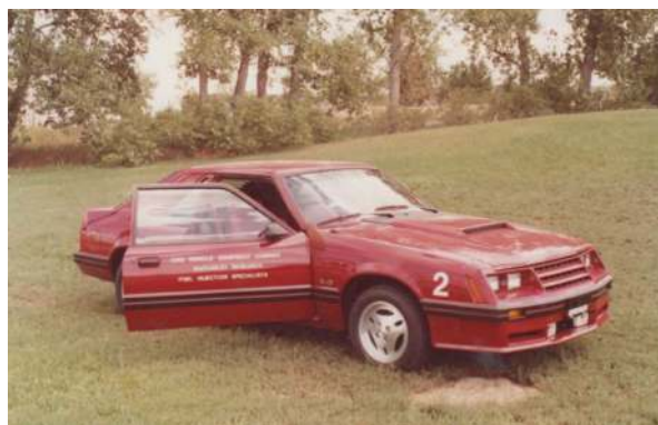
Fig. 8.11 1982 natural gas fuel-injected, turbocharged automobile constructed by author for evaluation of CNG fuel by Colorado State Agencies, 1982
