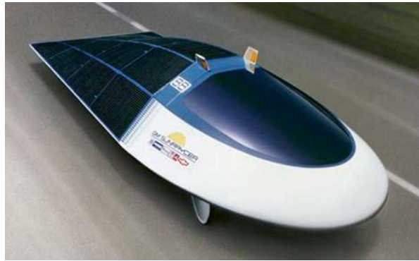
Fig. 5.2 General Motors Sunraycer, winner of Sun Race Australia, 1987. Solar cells occupied much of the surface area of the vehicle. (Creative Commons CC0)
