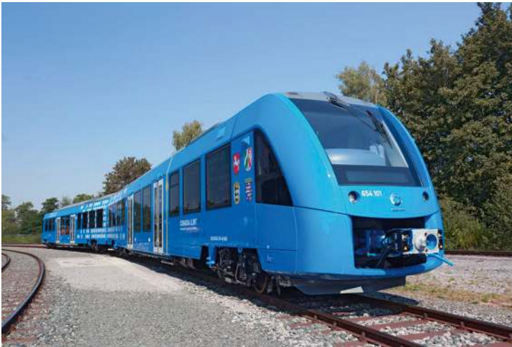
Fig. 9.28 The Coradia iLint, the first fuel cell hydrogen commuter train, shown in service in the Lower Saxony region of Germany, 2023. From https://cdn.railuk.co/wp-content/uploads/2016/09/24120435/IMG_5056_iLint_D-1068x712.jpg UK government agency, public domain
