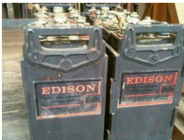
Fig. 14.9 Retro Nickel-iron batteries briefly produced 1972-75 by Exide Technologies, last owner of Edison Storage Battery Co., CC-BY SA Image by “Z22”, Wikipedia Free Repository
