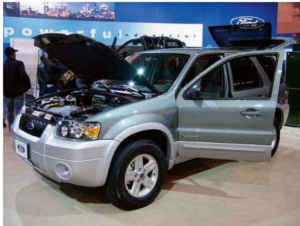
Fig. 15.21 The 2005 Ford Escape was the first hybrid car from a US manufacturer. It was also the first E85 hybrid. It utilized a power-split hybrid drive partially licensed from Toyota. Photo by Aude, 27 January 2006, at Washington Auto Show. Creative Commons Attribution-Share Alike 2.5 Generic license
