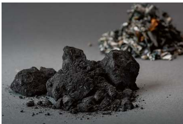
Fig. 14.63 “Black mass” from shredded lithium-ion batteries. Source: Argonne National Laboratory. Public domain
