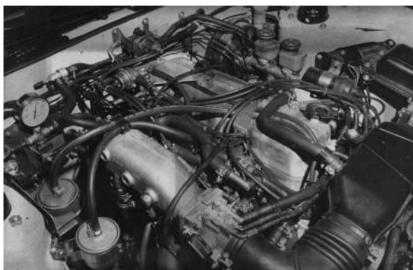
Fig. 6.11 Engine of 1981 DRI/DOE Multi-fuel Demonstration Vehicle showing dual-fuel injection systems. (Photo: author)
