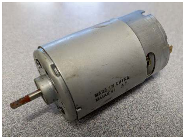
Fig. 14.38 Mabuchi 3T brush-commutated permanent magnet DC actuator motor. Permanent magnet design makes motor reversible by change in polarity. Photo: author
