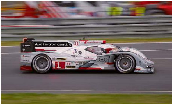
Fig. 15.26 A technical miracle: The Audi R-18 e-Tron diesel -electric hybrid that used a flywheel-electric accumulator for electric energy storage, winning the 24 Heures du Mans 2012–2014. Lithium batteries replaced the flywheel electric storage system in 2016, but by then, most other teams also fielded advance hybrids that used lithium batteries. Photo by kevinmcgill, 22 June 2013. Creative Commons Attribution-Share
