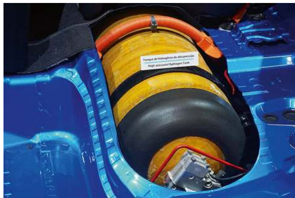
Fig. 9.34 Composite high-pressure hydrogen tank in Toyota Mirai. Photographer: Mario Roberto Duran Ortiz, 2016. https://commons.wikimedia.org/wiki/File:Toyota_Mirai_high-pressure_hydrogen_tank_SAO_2016_9036.jpg . Wikimedia Commons CC-BY-2.0
