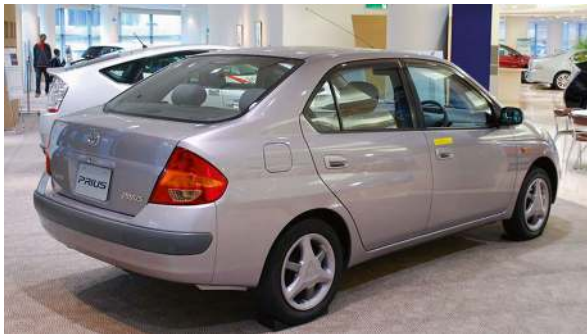
Fig. 15.20 1997 Toyota Generation 1 Prius, first mass market hybrid but sold only in Japan until 2002. Note right-hand-drive for Japanese market only. A power-split strong hybrid with a 35 kW electric drive motor. https://commons.wikimedia.org/wiki/File:1997_Toyota_Prius_01.jpg . Creative Commons Attribution-Share Alike 3.0 Unported, 2.5 Generic license CC BY-SA 3.0
