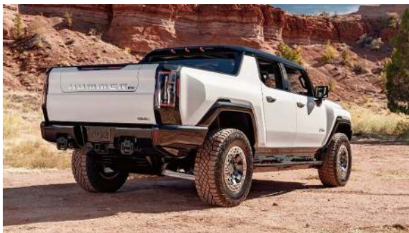
Fig. 14.67 2023 GM Hummer Electric pickup truck. At approximately 4350 kg (9600 lbs) curb weight, the heaviest and least efficient EV ever sold to the general public. The lowest range battery alone weighs 1326 kg (2923 lbs), which is more than the weight of most gasoline cars. MSRP from $87,000–$110,000 USD depending on trim and battery capacity, but since its release in December 2021, dealer markups have increased the selling price by an additional $50,000–$140,000 USD. https://www.gmc.com/electric/hummer-ev/pickup-truck
