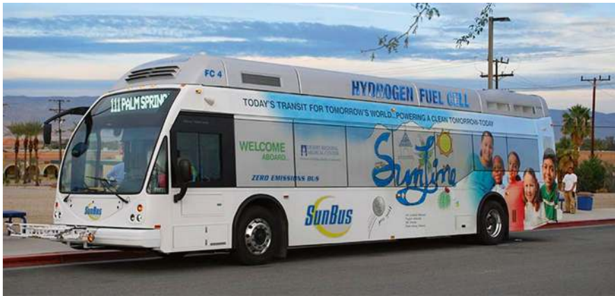
Fig. 9.27 Transit bus equipped with hydrogen fuel cell drivetrain produced by American Fuel Cell Inc. operating in Palm Spring, California, 2019. Photo by Leslie Eudy, NREL. https://www.nrel.gov/state-local-tribal/blog/posts/fuel-cell-electric-buses-in-the-usa.html . Public domain
