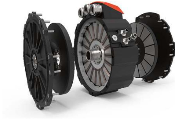
Fig. 14.41 CAD rendering of an axial flux EV motor from Magnax BV of Belgium, 2023. Larger in diameter but shorter in length than a conventional ECPM DC motor with similar ratings. https://spectrum.ieee.org/media-library/eyJhbGciOiJIUzI1NiIsInR5cCI6IkpXVCJ9.eyJpbWFnZSI6Imh0dHBzOi8vYXNzZXRxLnJibC5tcy8yNjc4NTM0MC9vcmlnaW4uanBnliwiZXhwaXJlc19hd-CI6MTY5MTI2NzA0MH0.MoS74fODyjc5TcjpinnHglC3DJO8hqxrb5uvmGplwJE/image.jpg . Creative Commons, CC BY-SA 4.0
