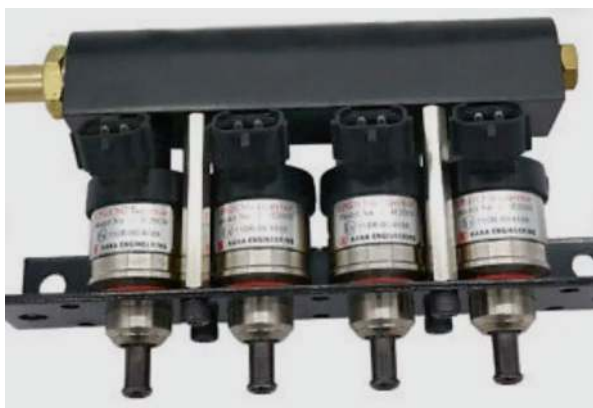
Fig. 4.19 Electrically actuated natural gas fuel injectors of the type used by Honda on the 1998–2015 Honda Civic GX NGV. Also used for custom CNG and LPG conversions. (Image: eBay. Public domain)
