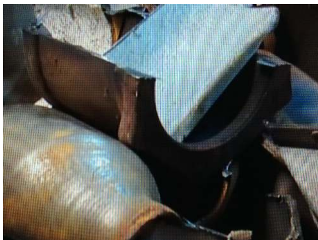
Figure 25.44 Cutaway sections of the scrapped metal casings from the substrates of the catalytic converters.
