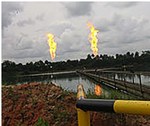
Figure 24.45 Flaring of associated gas from an oil well site in Nigeria (Source: www.en.m.wikipedia.org ).
