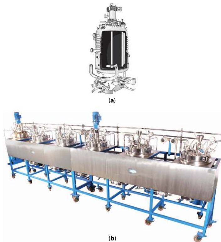
Figure 7 (a) Continuous stirred tank reactor with different impeller types. (b) A series of continuous-flow stirred tank reactors.
