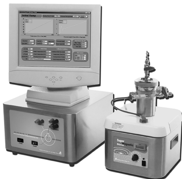
Figure 23.43a The Advanced Reactive System Screening Tool™ (ARSST™). (By permission from Fauske and Associates, Inc.)
