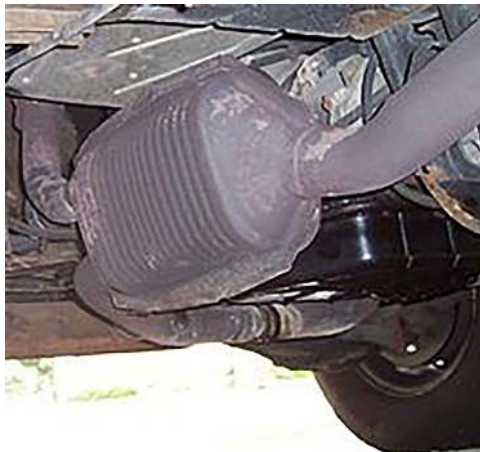
Figure 25.32 A three-way catalytic converter on a gasoline powered vehicle (Source: www.en.m.wikipedia.org ).
