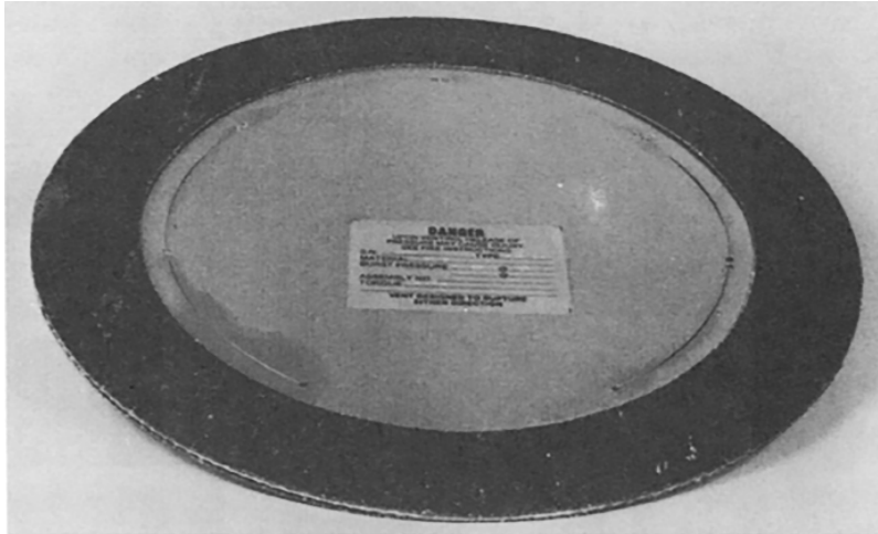
Figure 23.8i Flat disk used for low pressure and for isolation of corrosive environments. Usual pressure range is 2–15 psig with \pm 1 psi tolerance. Stainless steel disk with Teflon® seal usually standard. (By permission from Fike Metal Products Div., Fike Corporation. Catalog 73877-1, p. 35.)
