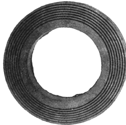
Figure 23.9a Non-metal frangible disk. Ruptured disk showing complete breakout of membrane. (Courtesy of Frails Industries, Inc.)
