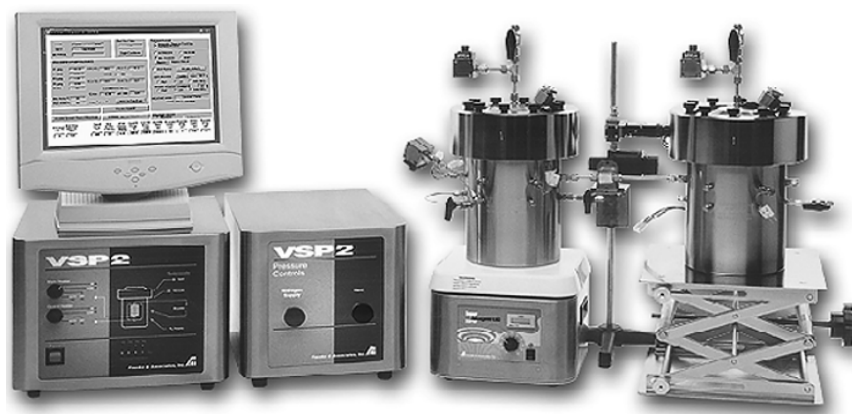
Figure 23.42 The Vent Sizing package 2™ (VSP 2™) apparatus. (By permission from Fauske and Associates, Inc.)
