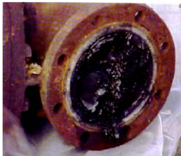
Figure 24.31 Blockage in valve C (Source: www.csb.gov).
