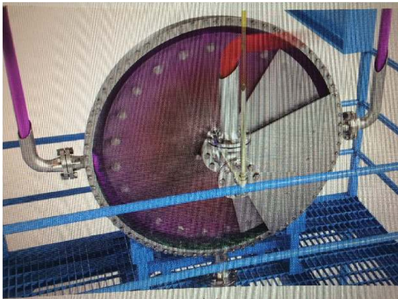
Figure 27.77 CycloneCC showing its operation with flue gas introduced on the left side and solvent at its center and the exit absorbed CO 2 gas (colored red) (Source: Carbon Clean Solutions Ltd.).
