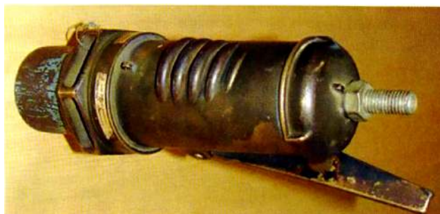
Figure 23.19a Relief valve installed horizontally. The markings on the bonnet result from the spring working its way out. (Source: Chris Flower and Adam Wills, The Chemical Engineer , U.K., pp. 24-31, June 2017.)
