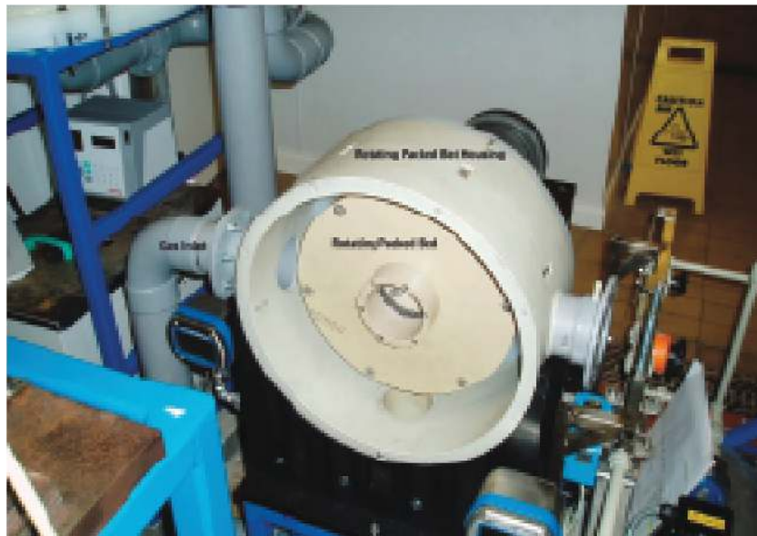
Figure 27.74b Laboratory scale rotating packed bed absorber (Source: GTI-ROTA – CAP: An Intensified Carbon Capture System Using Rotating Packed Beds).
