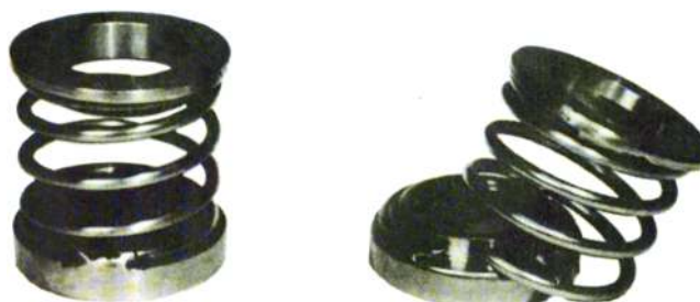
Figure 23.93 End caps welded to spring. Failure occurred at weld.
