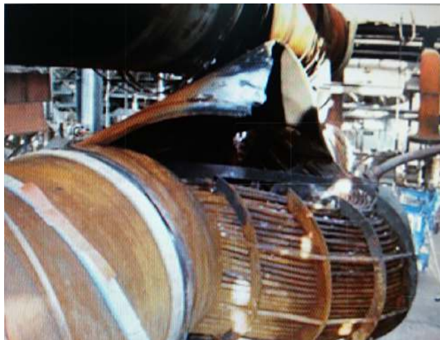
Figure 24.15 Close-up of ruptured heat exchanger (Source: www.csb.gov).
