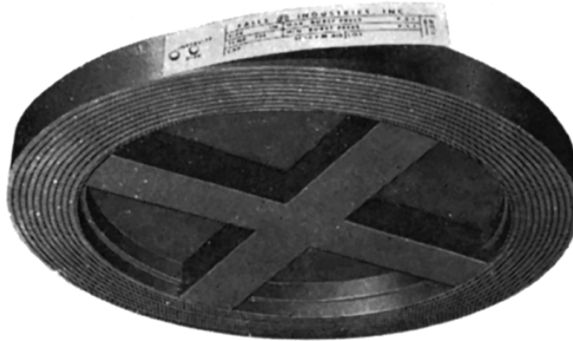
Figure 23.9f For pressure ratings of 15 psig or lower, subject to internal vacuum conditions, a vacuum support is required that is an integral part of the rupture disk and cannot be added in the field. (By permission from Falls Industries.)
