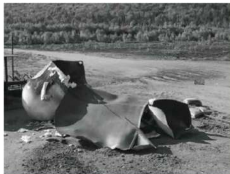
Vessel flattened on ground following BLEVE.
