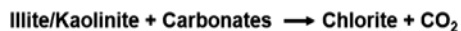
Figure 2.31 Mechanism for thermal decomposition of carbonates in argillaceous sandstone and shale. (As proposed by Smith and Ehrenberg (1989).)
