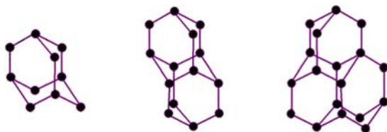
Figure 4.26 From left to right, the molecular structures (carbon skeletons) of adamantane, diamantane and trimantane, the smaller diamondoids, with chemical formulas C_{10}H_{16} , C_{14}H_{20} and C_{18}H_{24} , respectively. (From Mansoori (2007) .)
