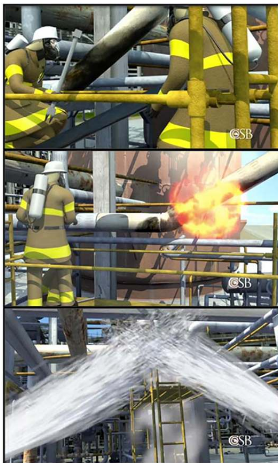
Figure 19.213 CSB animation of firefighters attempting to remove the 4-sidecut insulation, the resulting fire and fire extinguishing (Source: www.csb.gov ).
