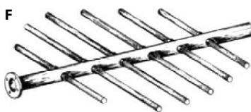
Figure 20.8F Typical design inlet liquid distributor using holes (orifices) on underside of distributor pipes. Note: Number of side pipes adjusted to provide uniform entry per square foot of water cross sectional area. Holes at wall should be spaced on the same basis.
