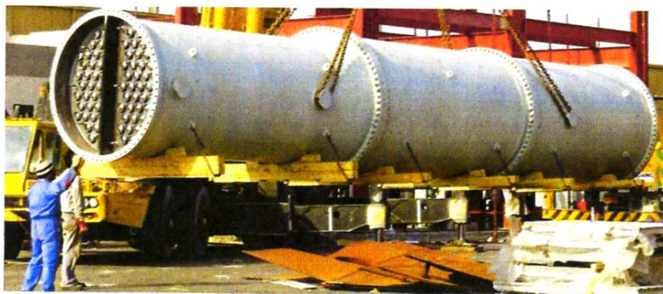
Figure 19.191 Cyclic distillation (dividing wall) column prepared for transportation to a chemical site (Source: Kiss, A., et al. [236]).
