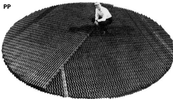
Figure 20.6PP Nutter Snap-Grid™ grid packing as assembled. Used by permission of Nutter Engineering, Harsco Corp. Bull. CSG-1.
