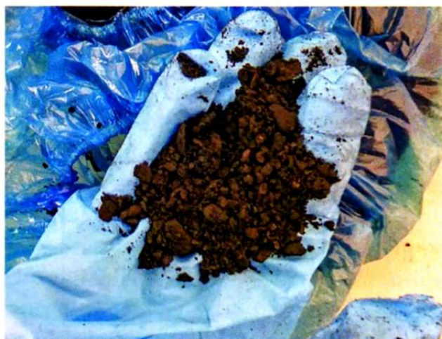
Figure 19.151 Accumulated fouling in the kerosene downcomer (Source: Ozturk, G., et al. Hydrocarbon Processing, Feb. 2021 [237]).
