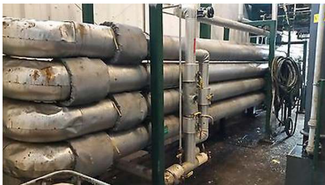
Figure 31 Plug flow reactor, 243' long, 8" S 40 CP pipe. A series of plug flow reactors.
