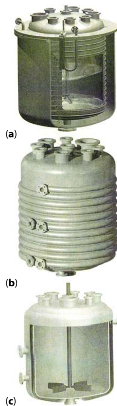
Figure 38 Batch reactor types with (a) constant flux (Coflux) jacket, (b) half coil jacket, and (c) a single external cooling jacket.
