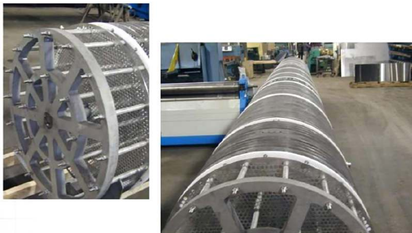
Figure 20.98C KARR® Column plate stack assembly (source: Koch Modular Process System (KMPS) LLC).
