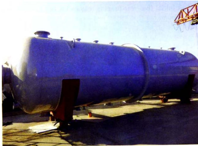
Figure 18.79 Photograph of a three-phase separator [84].
