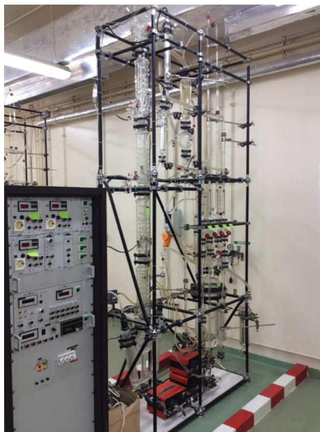
Figure 4.2 Laboratory distillation column with controls and accessories.
