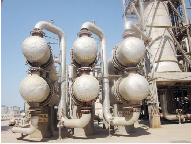
Figure 7.38 A photograph of kerosene hydrodesulfurizer reactor with feed/effluent shell and tube heat exchangers in series.
