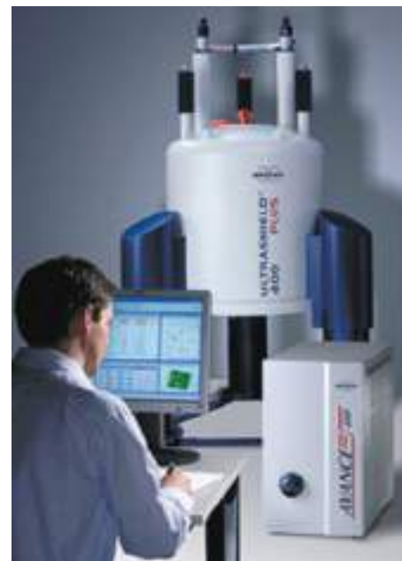
Photo of a 400-MHz NMR spectrometer. The metal container at the back contains the superconducting magnet, cooled by a liquid helium bath. The electronics used to control the spectrometer and to calculate spectra are at right.
