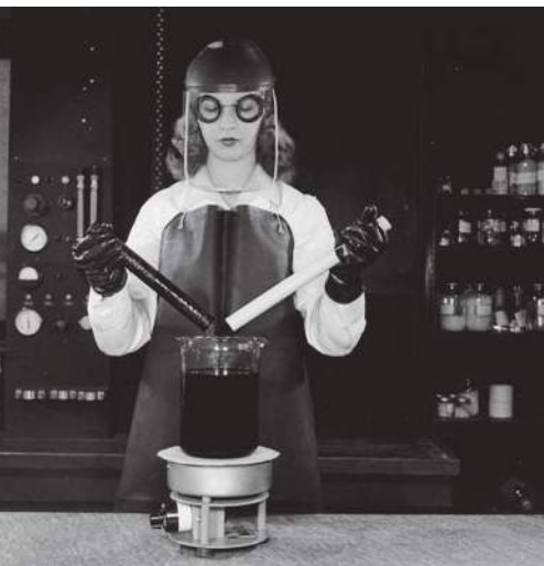
This 1949 DuPont promotional photo shows how a Teflon rod (on our right, in the model's left hand) resists a hot acid solution compared with a rod made from another plastic. In World War II, Teflon was used for insulation in aircraft wiring and for seals in the equipment used to enrich corrosive uranium hexafluoride.
