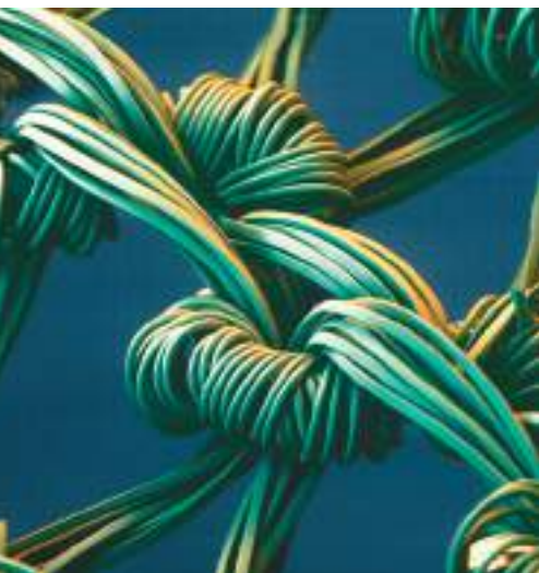
Scanning electron micrograph of the material in a nylon stocking. Sheer stockings require long, continuous fibers of small diameter and enormous strength. (Magnification 150X)
