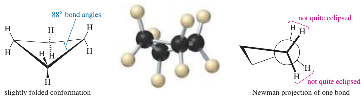
FIGURE 3-17 The conformation of cyclobutane is slightly folded. Folding gives partial relief from the eclipsing of bonds, as shown in the Newman projection. Compare this actual structure with the hypothetical planar structure in Figure 3-14.
