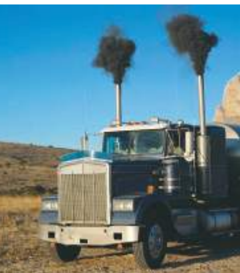
The black material in diesel exhaust consists of small particles that are rich in polynuclear aromatic hydrocarbons.
