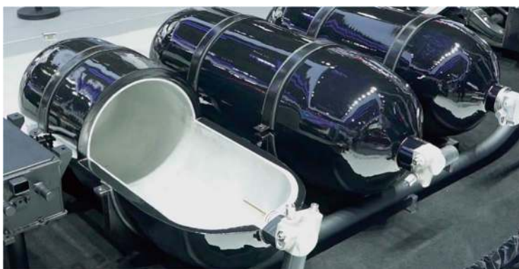
Fig. 2.12 70 MPa carbon fiber wound aluminum alloy gas tank loaded on SAIC Maxus EUNIQ7
