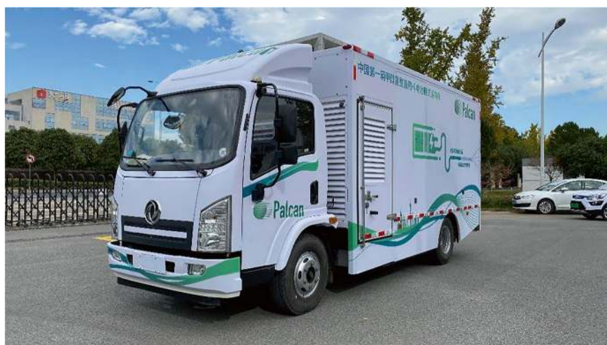
Fig. 4.25 The world's first light-duty truck based on methanol reforming hydrogen fuel cells, jointly produced by Dongfeng Special Vehicle Co., Ltd. and Suzhou Qingjie Power Supply Technology Co., Ltd.
