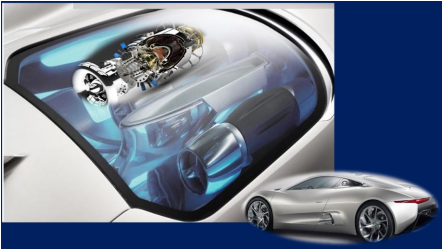
Fig. 10.6 Jaguar C-X 75 with two gas turbines for power generation on board and four electric motors (one per wheel) for propulsion
