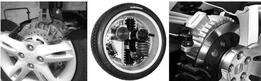
Fig. 13.2 Wheel hub motors for vehicle drive: Mitsubishi (left), Michelin (middle), Honda (right) (Sources: Mitsubishi, Michelin, Honda)
