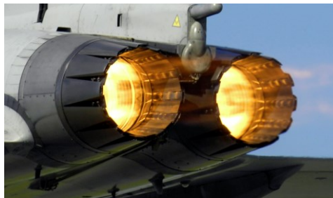
Fig. 7.5 Exhaust gas flow through the nozzles of the jet engines of an aircraft (Source: Eurofighter Typhoon F2, RAF)
