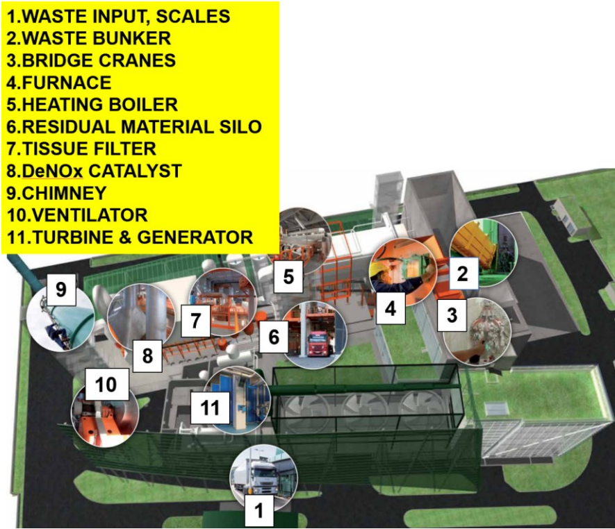
Fig. 14.2 Combined Heat and Power Plant with waste burning in Bolzano/Italy – functional schematic (Source: ECO Center AG, Bolzano)
