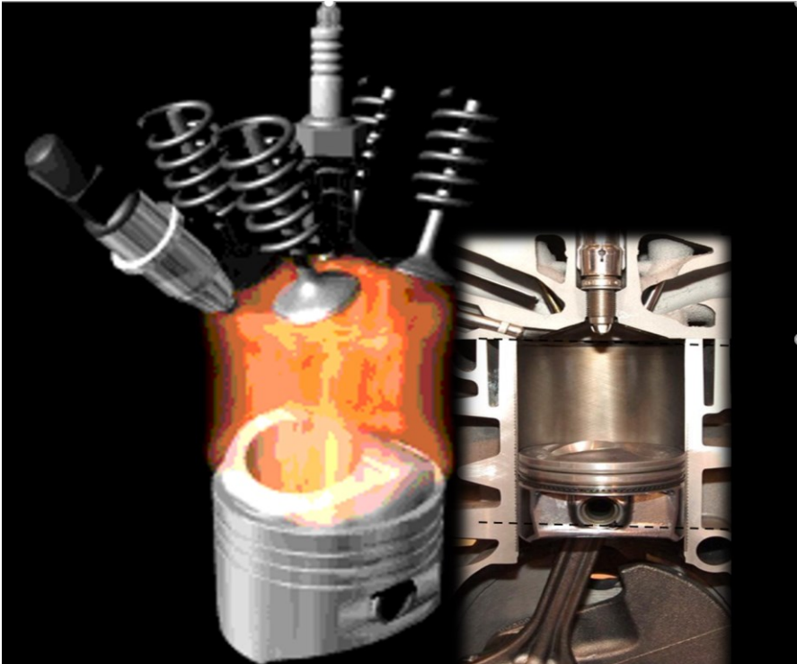
Fig. 3.4 During combustion, the temperature of the burned gas mixture formed in the combustion chamber of a piston engine increases. As a result, the pressure in the mixture increases, which pushes the piston
