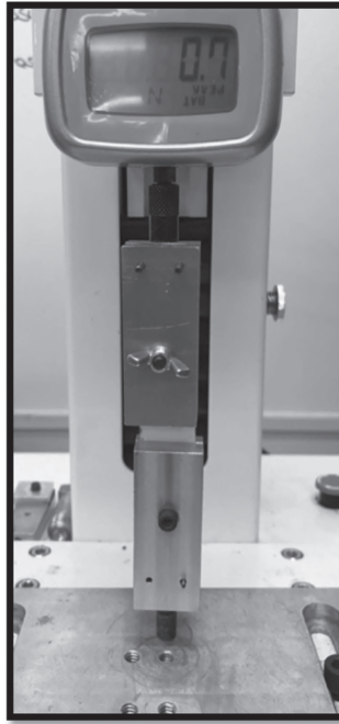
FIGURE 10.8 Polyimide–SiO 2 nanocomposite undergoing tensile testing—mechanical characterization. Source: Based on [30].
