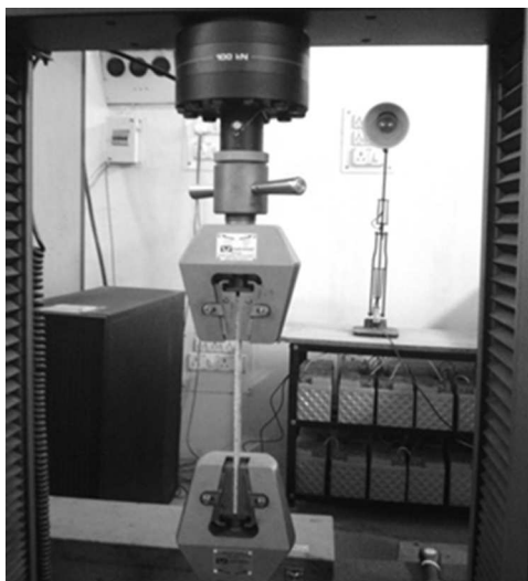
FIGURE 7.2 ASTM D-3039 testing system setup.
