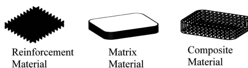
FIGURE 1.3 Fabrication of composite material with a reinforcing phase and matrix phase.
