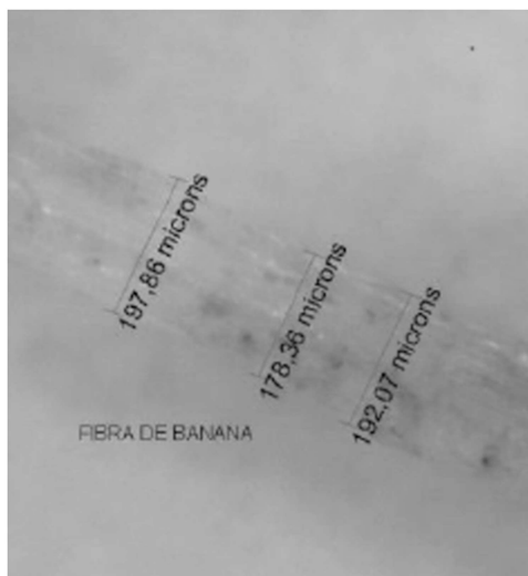
FIGURE 3.6 Optical micrograph of banana fiber (Vasconcelos et al., 2014).
