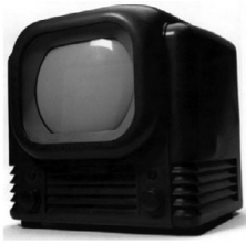
Figure 1.3 Phenolic composite (Bakelite) application: the casing of an early mass-produced TV (1953).
