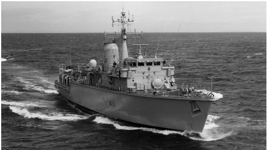
Figure 1.2 GRP minesweeper: an example of scale-up of early techniques for larger ships.
