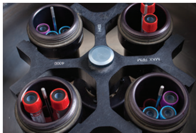
Figure 1.12 Properly loaded centrifuge.
