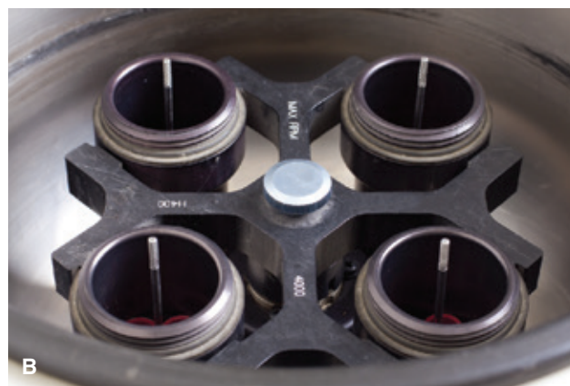
Figure 1.10 (A) Benchtop centrifuge. (B) Swinging-bucket rotor.
