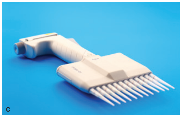
Figure 1.6 (A) Adjustable volume pipette. (B) Fixed volume pipette with disposable tips. (C) Multichannel pipette. (D) Multichannel pipette in use.
