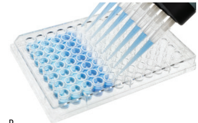
Figure 1.6 (A) Adjustable volume pipette. (B) Fixed volume pipette with disposable tips. (C) Multichannel pipette. (D) Multichannel pipette in use.
