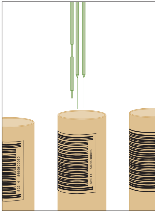
Figure 5.4 Dual sample probes of a chemistry analyzer. Note the liquid-level sensor to the left of probes.
