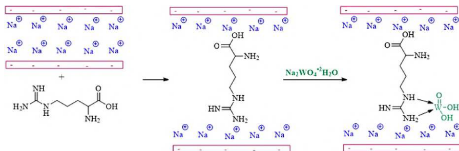
SCHEME 2.40. The preparation of bentonite@ L-arginine-WO 3 .
