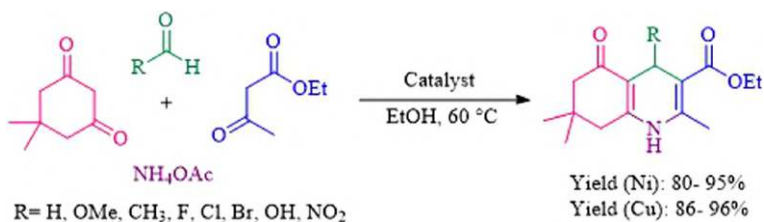
SCHEME 4.12. Application of Ni and Cu embedded on SBA-15 decorated with glycine for the synthesis of polyhydroquinolines.
