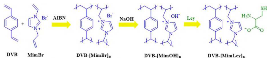
SCHEME 3.33. Ionic copolymers DVB-[MimLcy] n preparation pathway.
