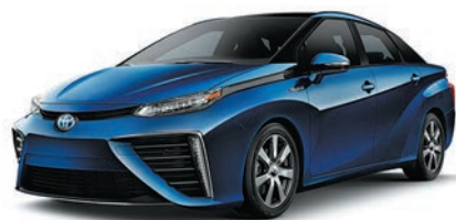
▲ FIGURE 16.1 A fuel-cell car The Toyota Mirai is the first mass-produced fuel-cell vehicle. It is powered by hydrogen and its only emission is water.
