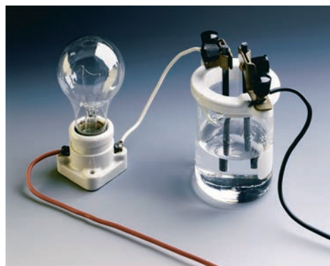
▲ FIGURE 14.12 Conductivity of a weak electrolyte solution
