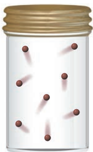
▲ FIGURE 11.7 A gas assumes the shape of its container Since the attractions between molecules in a gas are negligible, and since the particles are in constant motion, a gas expands to fill the volume of its container.
