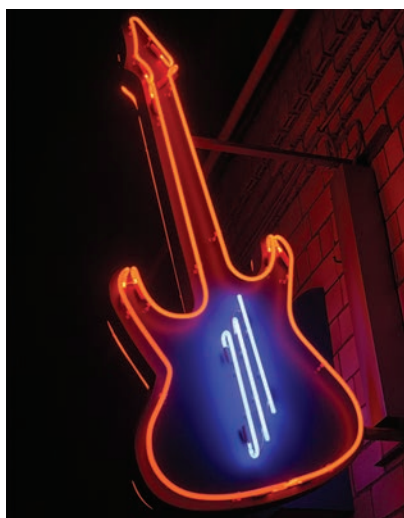
▲ FIGURE 9.6 A neon sign Neon atoms inside a glass tube absorb electrical energy and reemit the energy as light.
