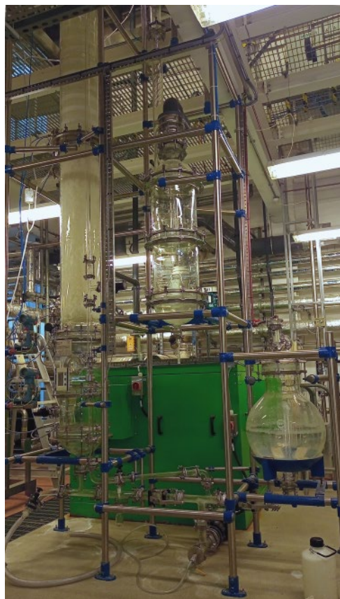
Figure 20.3 Approx. 4 m pilot-scale absorption column based within the Department of Chemical Engineering at the University of Manchester.
