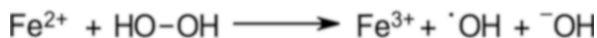
Fig. 12.1 The Fenton reaction. In the presence of hydrogen peroxide, ferrous iron ( \text{Fe}^{2+} ) is readily oxidized into ferric iron ( \text{Fe}^{3+} ), forming both a hydroxyl radical and a hydroxide ion in the process. Hydroxyl radicals can lead to harmful and deleterious oxidation of biomolecules if uncontrolled
