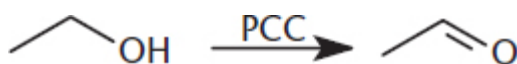
Figure 5.6 Oxidation of a Primary Alcohol to an Aldehyde by Pyridinium Chlorochromate (PCC)
