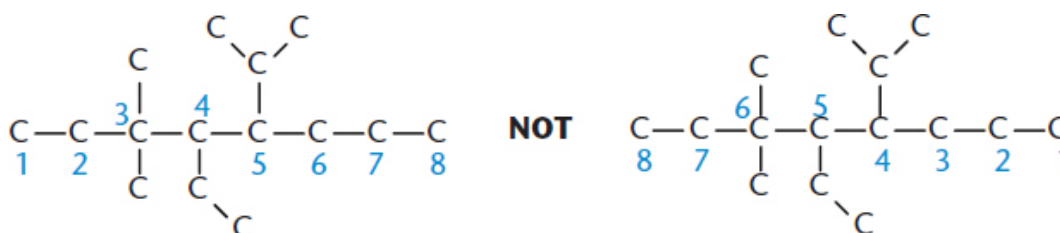
Figure 1.2 Numbering the Longest Carbon Chain The highest-priority functional group should have the lowest possible number; if all substituents have the same priority, as in this figure, make their numbers as low as possible.
