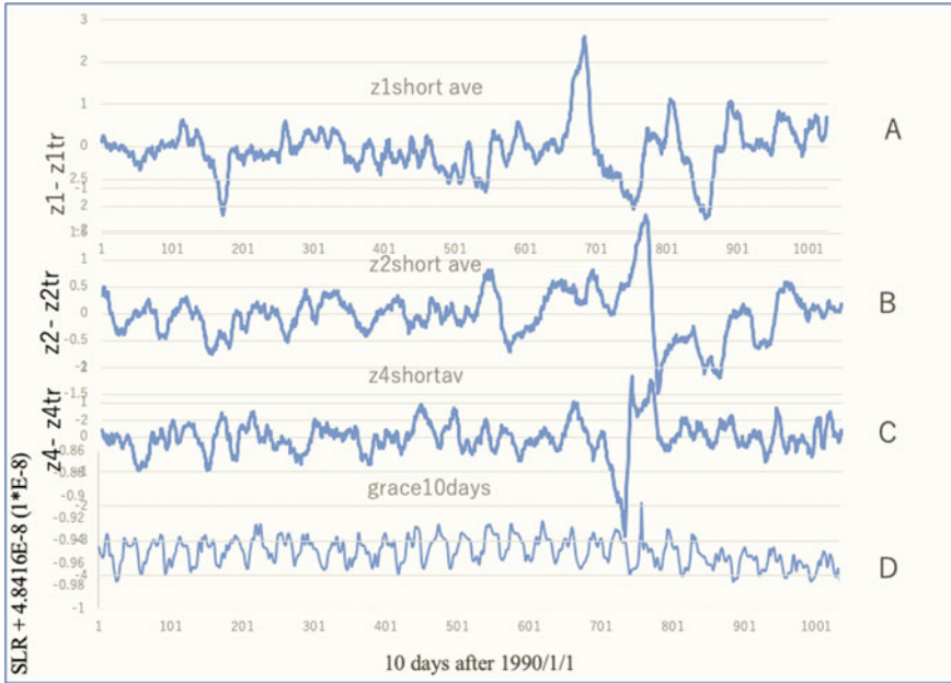
Fig. 5.15 Comparison of the temporal variations among short-term z_1 , z_2 , and z_4 of the global correlated seismicity and sea level rise (SLR) from satellite observation showing the different periodicity and phase shift between them
