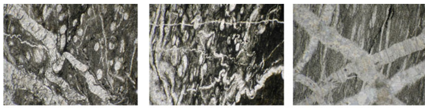
Fig. 2.18 Microphotographs of metamorphic chert thin sections showing the plastic deformation of sealed open cracks and quartz-filling radiolarian fossils in various degree of strain. See sharp cut of the quartz-filling fossils by deformed sealed open crack. Notice that the chert is almost always composed of fine-grained quartz as well as open crack and fossils. Bar represents 0.1 mm
