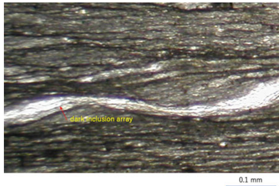
Fig. 2.3 Illustration of open crack and shear crack geometry with jog, showing elongated growth direction of sealing minerals and the examples of natural occurrence
