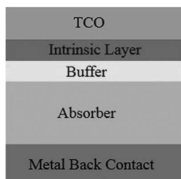
FIGURE 14.3 Physical structure of chalcogenide solar cells.
