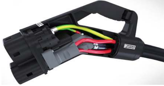
Fig. 18 Interior of connector reveals its intricate design, featuring AC cables (green) and a liquid cooling system for the DC cables (red). ( Image Phoenix Contact )
