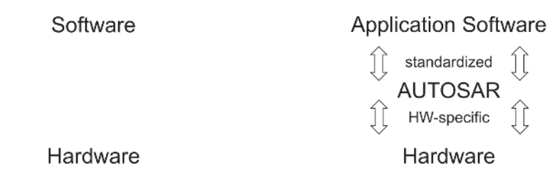
Figure 4. Legacy SW and AUTOSAR-based SW implementation [25].
