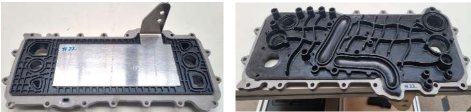
Figure 20. Plastic-intensive MPP after compression molding; stack side (left) and MIU side (right).
