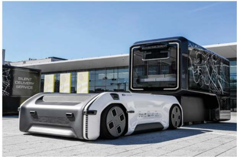
Figure 1. Driveboard (on the left) drives up to passenger capsule (on the right) [1].
