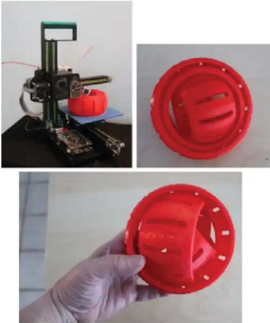
Figure 4. Examples of print moveable parts as a single piece [17].
