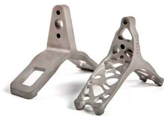
Figure 2. Examples of design topology optimization: The final ENDY additive bracket part (left) weighs about 40% less than the original (right), weighing in at 152 g instead of 250 g [15].
