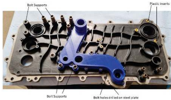
Figure 21. Plastic-intensive MPP after bolt supports and inserts were pressed.
