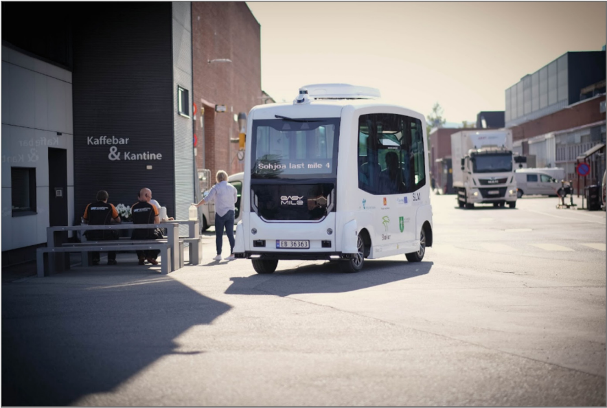
Fig. 2. The autonomous shuttle, driving without any adaptation in infrastructure such as road/guiding markings
