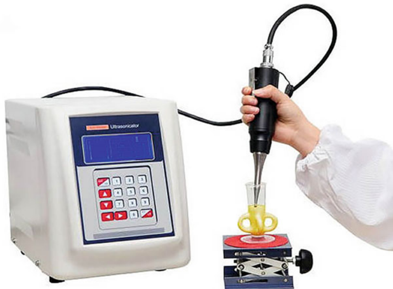
Fig. 1 Perform sonicating cell lysate. Sheared with 4–5 sets of 10-second pulses on wet ice
