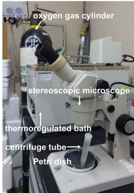
Fig. 2 Instruments and arrangements for the dissociation of adrenal medullary cells. The adrenal cortex is removed from the adrenal gland under microscopic observations in a Petri dish whose bottom is covered with silicone mixed with carbon powder. O 2 gas is delivered through a polyethylene tube from an O 2 gas cylinder to the bottom of a centrifuge tube that is filled with 1.5 mL of collagenase-containing Ca 2+ -free balanced salt solution
