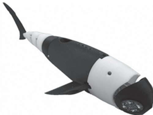
FIGURE 10.4 Fish robot body (Waduge and Joordens, 2017).
