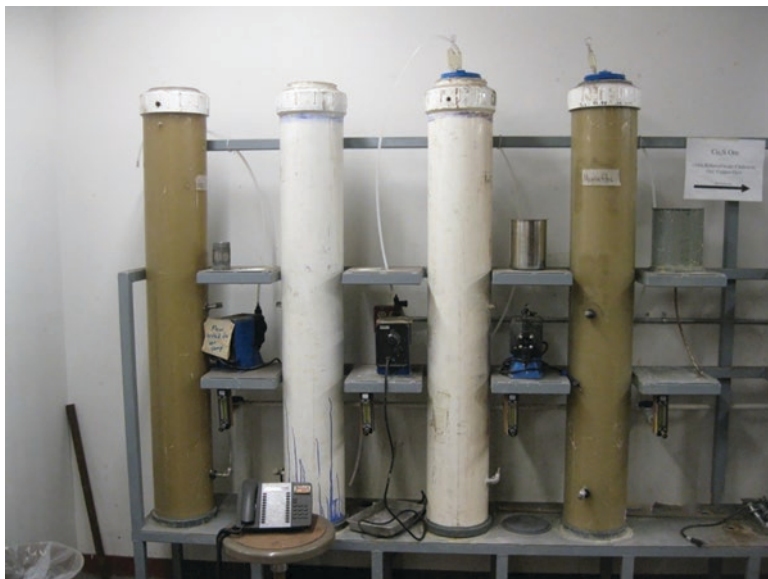
Fig. 4 Medium-size column bioleaching setup (50 kg capacity each)
