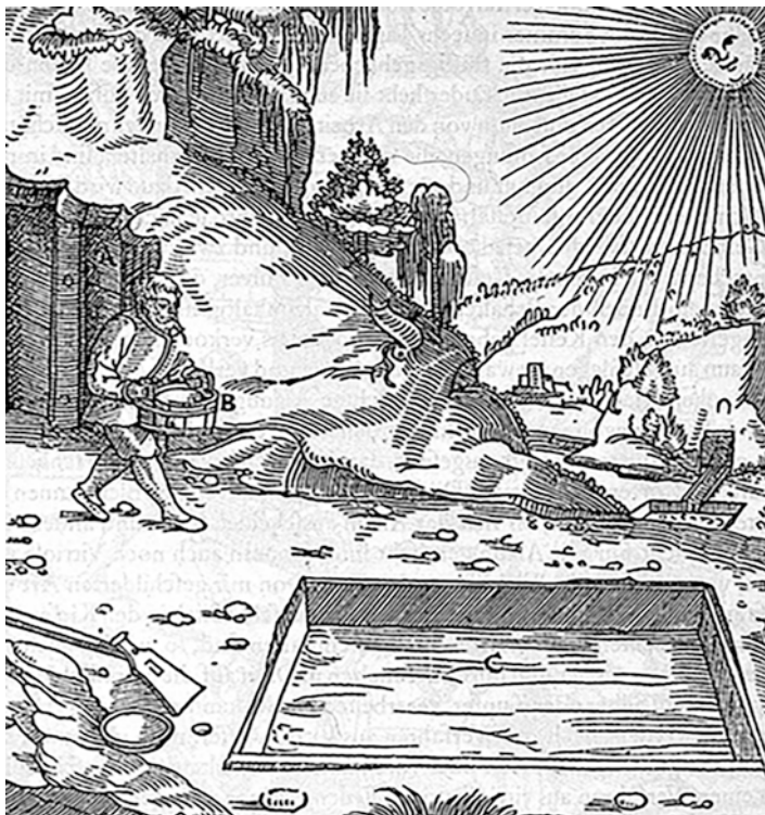
Fig. 1 Woodcut from the book de re metallica written by Georgius Agricola (1494–1555) illustrating the manual recovery of copper-containing mine effluents which are collected in wooden basins and concentrated in the sun
