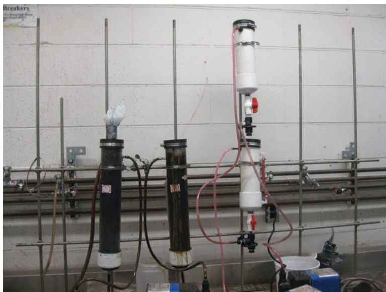
Fig. 3 Small-scale bioleaching column (2 kg capacity)
