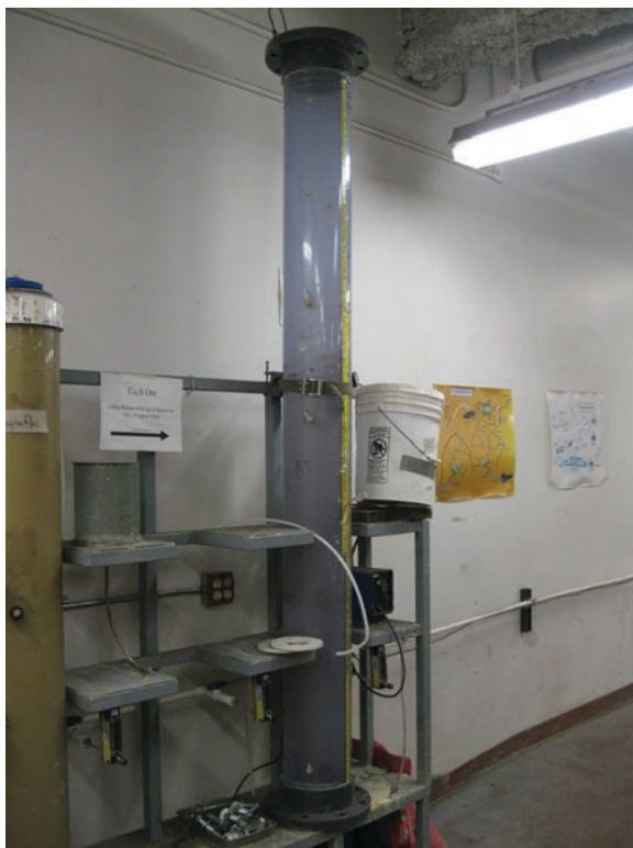
Fig. 4 Medium-size column bioleaching setup (50 kg capacity each)
