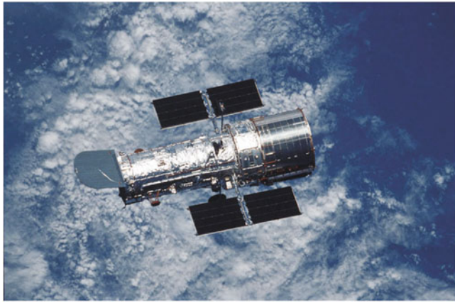
Fig. 5.14 The space telescope (Hubble Space Telescope). You can see the two Stretched out solar cell arrays as well as the open protective flap. NASA/ESA
