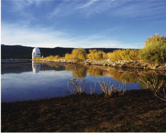
Fig. 5.8 Big Bear Solar Observatory in California, USA. The water surface has a calming effect on air turbulence
