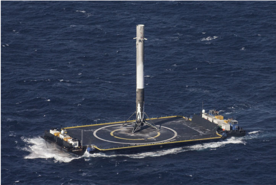
Fig. 4.12 The landed burned out rocket stage of Falcon (SpaceX Photos)
