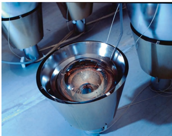
Fig. 5.7 The photomultiplier's "eye" is visible in the image. Inside the photomultiplier, a metal photocathode absorbs incoming photons and emits electrons. These electrons are then multiplied through a cascade of dynodes until they reach an anode, which generates an electrical pulse. During the electron multiplication process, the electrons can be deflected by the Earth's magnetic field. To prevent this, a cylinder made of "mu-metal" is mounted around the photomultiplier, effectively shielding it from the Earth's magnetic field
