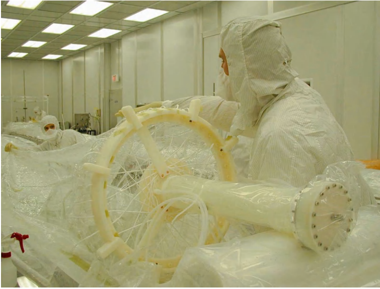
Fig. 5.9 The clean room at Princeton, where the nylon was extruded, the material assembled, and the IV (surrounded by the OV) was constructed; it is equipped with a cryogenic system to eliminate radon. Operators wear clean uniforms and masks to isolate themselves from the environment and prevent contamination of the room. It is worth noting that human breath is one of the primary sources of contamination in clean rooms
