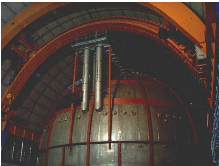
Fig. 5.6 Again the external tank (water tank). In this photo, which shows the upper part of the tank, you can see the so-called organ pipes through which the cables of the photomultipliers mounted inside come out. There are eight pipes in total
