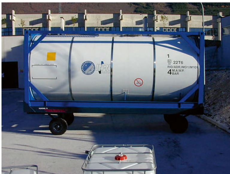
Fig. 5.12 An Isotank for transporting Pseudocumene. It is a container designed for transporting liquid or gaseous products, such as fuel, chemicals, cement, or tar. It must meet specific requirements, including a certain wall thickness, suitability for internal pressurization, maximum sealing, and other safety and performance standards. In our case, the isotank was also specially treated internally, similar to the other containers used for our scintillator. It underwent four different surface treatments to extract contaminants embedded in the material and to facilitate the removal of dust and particulates
