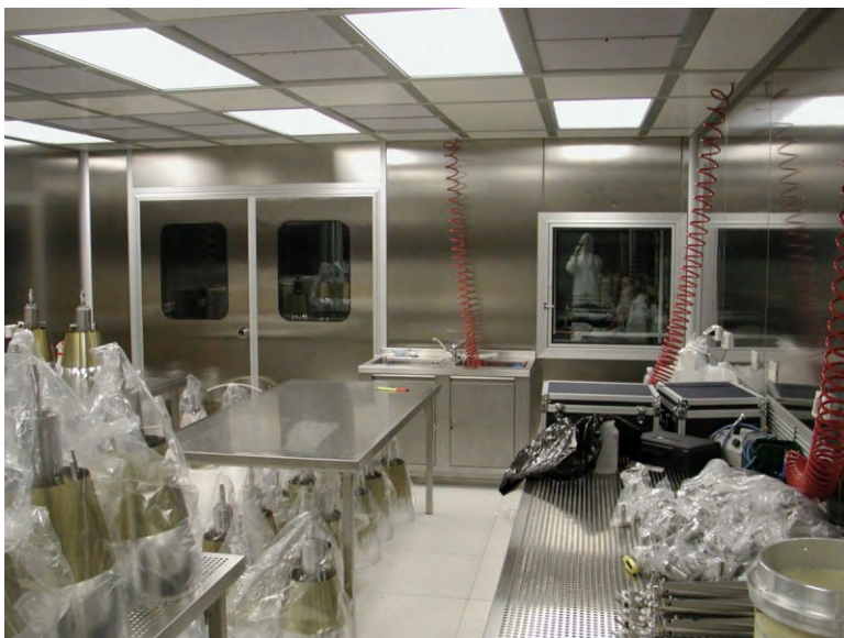
Fig. 6.1 Photomultipliers equipped with optical concentrators and encased in mu-metal, meticulously cleaned and double-bagged within the clean chamber located at the inlet of the detector water tank
