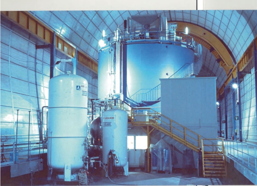
Fig. 4.2 The external tank of the CTF, a large cylindrical structure, is shown installed in Hall C of the underground Gran Sasso Laboratory. Positioned at the center of the hall, the tank features various control and monitoring systems on its upper section. Among these is a continuous recording system for measuring radon levels in the hall's atmosphere. Additional systems visible in the photo are auxiliary components essential for operating the CTF. These are not described here, as delving into their technical details might overwhelm the reader. Hall C itself is an impressive space: 30 m wide, 30 m high, 100 m long. It is lined with aluminum panels and equipped with a large, movable scaffolding system. This scaffolding, combined with an overhead crane, facilitates the transportation of heavy equipment throughout the hall
