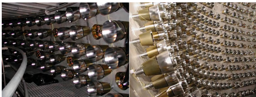
Fig. 6.6 On the left, a close-up of the photomultipliers installed with the scaffolding still in place; on the right, a section of the sphere with the photomultipliers fully installed. (The photo on the right was reproduced on the 2014 commemorative stamp of the Italian Post Office)
