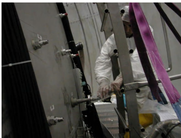
Fig. 6.10 An operator, positioned outside the sphere, is testing the airtightness of the terminal section of the photomultipliers, which pass through the sphere and extend into the water tank. The seal must be 100% airtight; if air and vapors cannot pass through, we can be confident that liquids, such as pseudocumene and water, will also be effectively sealed. This test was performed on all the photomultipliers using a portable mass spectrometer
