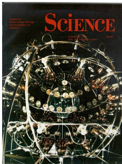
Fig. 4.3 The internal structure of the CTF photographed by a camera inside the external tank. You can see the nylon container of the scintillator, the structure with the photomultipliers mounted and the relative cables. This is the cover of a 1994 issue of the scientific journal Science . (Source: Science , License number OP-00165285, License date 20 December 2024). This image was also featured on the cover of the German magazine Naturwissenschaften in 1997 and the Hungarian magazine Természet Világa in 1996
