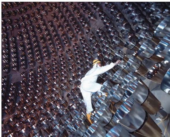
Fig. 6.9 Paolo Lombardi is addressing an issue with an optical fiber that was not properly transmitting the laser pulse to the photomultiplier
