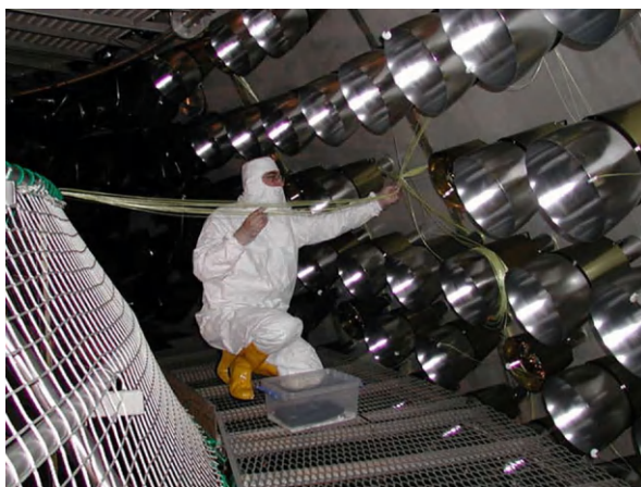
Fig. 6.8 Lino Miramonti is connecting the optical fibers to the individual photomultipliers for continuous gain monitoring. The fibers transmit light pulses, generated by a connected laser, to the photomultipliers
