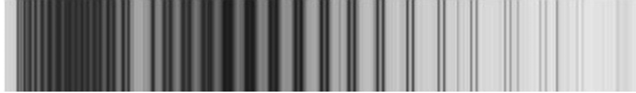
Figure 2.11 Telluric Fraunhofer A molecular absorption spectrum generated by sunlight [1]
