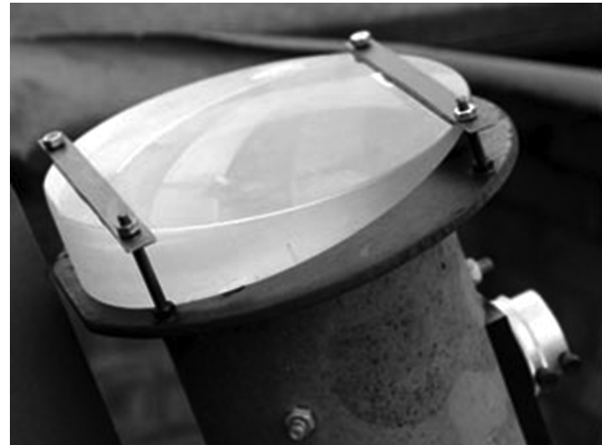
Figure 4.8 Objective prism (21 cm diameter, 50 to 5 mm thickness slope, 12^\circ tilt angle) mounted on top of an 11 cm f/5 Newtonian telescope.
