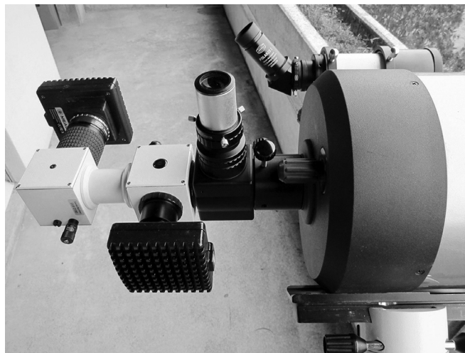
Figure 6.7 The spectrograph, an additional load to the mount
