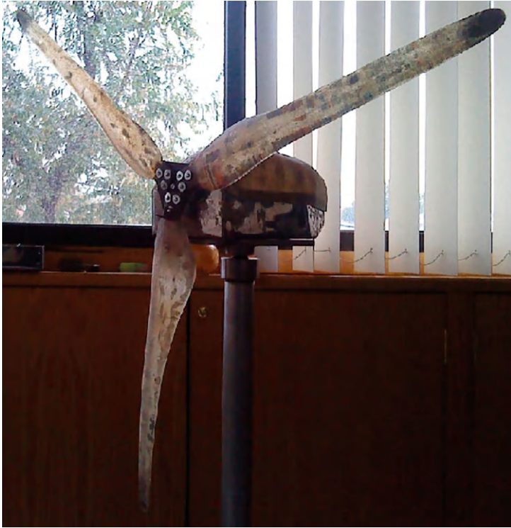
Fig. 4.4 Prototype of the manufactured wind turbine
