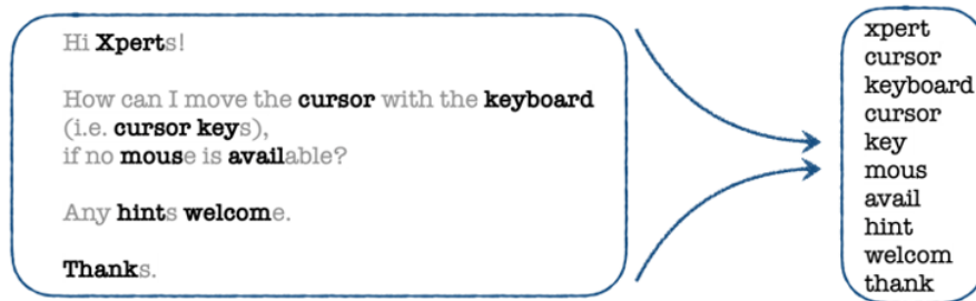
Figure 10.11 Preprocess function allows you to considerably reduce the dimensionality of your original feature space: it converts all words to lowercase, removes punctuation marks, stopwords and words shorter than 4 characters, and outputs a list of stems for the remaining words.
