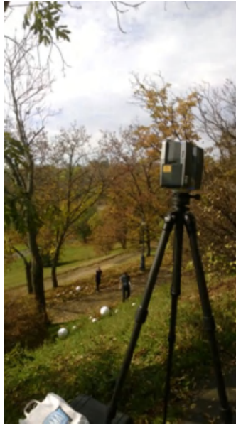
Fig. 4.62 The scanner at the top of the measured steep slope with the different sizes of white spheres as control points in the background
