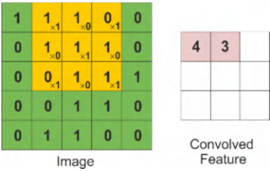
Fig. 5.88 Illustration of convolution process. Considering the multiplication and summation of the corresponding image and convolution filter elements, i.e
