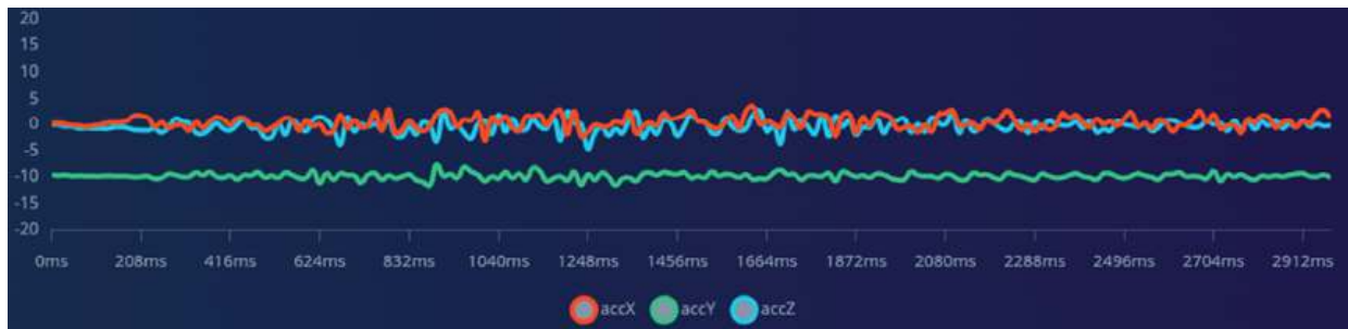
Figure 3.11: Sample of acceleration readings during correct drilling
