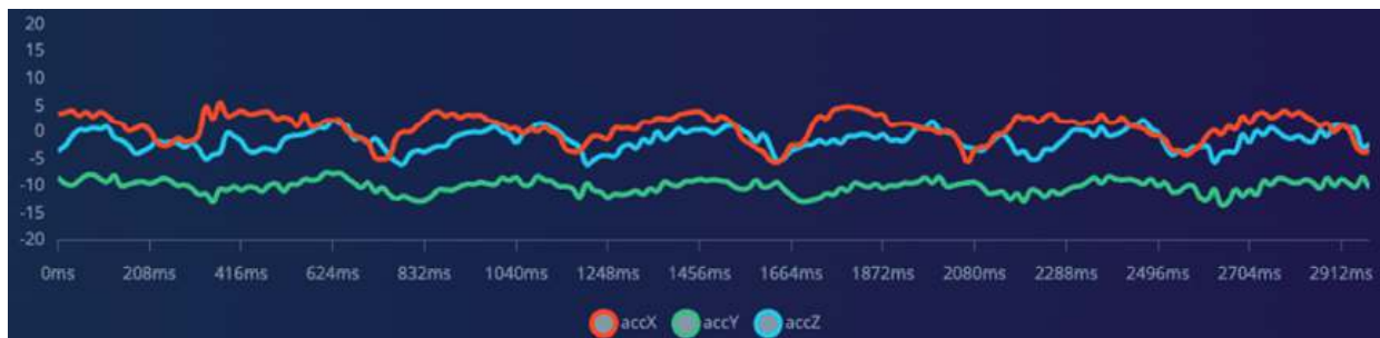
Figure 3.12: Sample of acceleration readings during incorrect drilling
