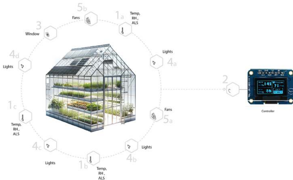
Figure 7.6: Concept diagram (Greenhouse control)
