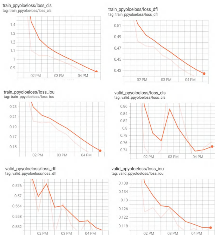
Fig. 4 Training and validation losses for a YOLO-NAS object detection model. The graphs show that both the training and validation losses decrease over time
