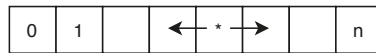
Figure 3. The Corridor environment. The agent (denoted by “*”) is inserted randomly and its goal is to reach the final state n by executing two actions—moving left or right.
