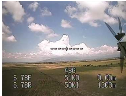
Figure 1. Captured image of a video stream from a camera mounted on an unmanned aerial vehicle (UAV). The image resolution is 720 width and 480 height at a 30 frames per second.
