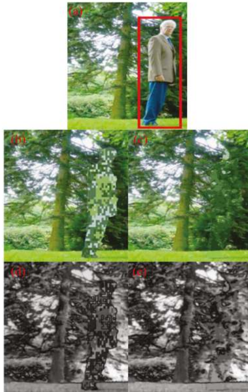
Figure 13. Comparison between our method and an existing method. (a) original image; (b) traditional camouflage texture; (c) adaptive camouflage texture; (d) the saliency map corresponding to image (b); (e) the saliency map corresponding to image (c).
