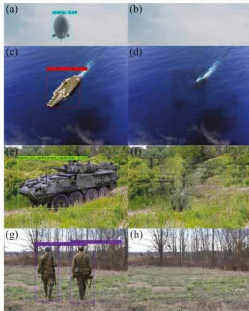
Figure 10. More detailed experimental results. (a) airship; (b) preliminary camouflage texture of the airship; (c) aircraft carrier; (d) preliminary camouflage texture of the aircraft carrier; (e) tank; (f) preliminary camouflage texture of the tank; (g) uniformed soldiers; (h) preliminary camouflage texture of the uniformed soldiers.
