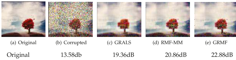
Figure 6. The Results of Image recovery with salt-and-pepper noise.
