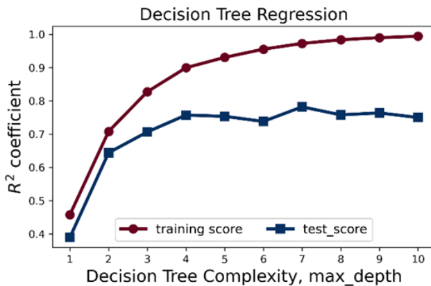
Figure 1.5 Comparing decision trees of different depths on the Boston Housing regression data set using R^2 as the evaluation metric. Higher R^2 scores mean that the model achieves lower error. An R^2 score close to 1 means that the model achieves nearly zero error.
