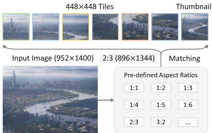
Fig. 2.5 Illustration of dynamic high resolution. We dynamically match an optimal aspect ratio from pre-defined ratios, dividing the image into tiles of 448 \times 448 pixels and creating a thumbnail for global context. This method minimizes aspect ratio distortion and accommodates varying resolutions during training
